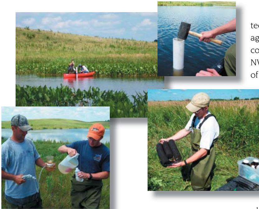
*A short, light canoe (upper left) worked well to access the open water zone of wetlands from which to collect samples of sediment (upper and lower right) and water (lower left) for analysis of several different types of pesticides, metals, and nutrients.*
