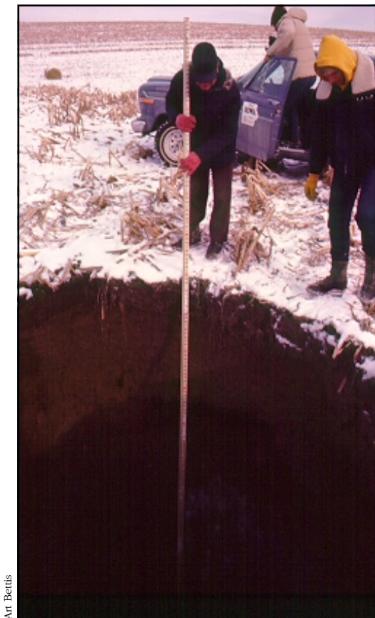
Figure 2. Measurements are made of a newly formed sinkhole, caused by collapse of soil and shallow rock into a subterranean cavern.
