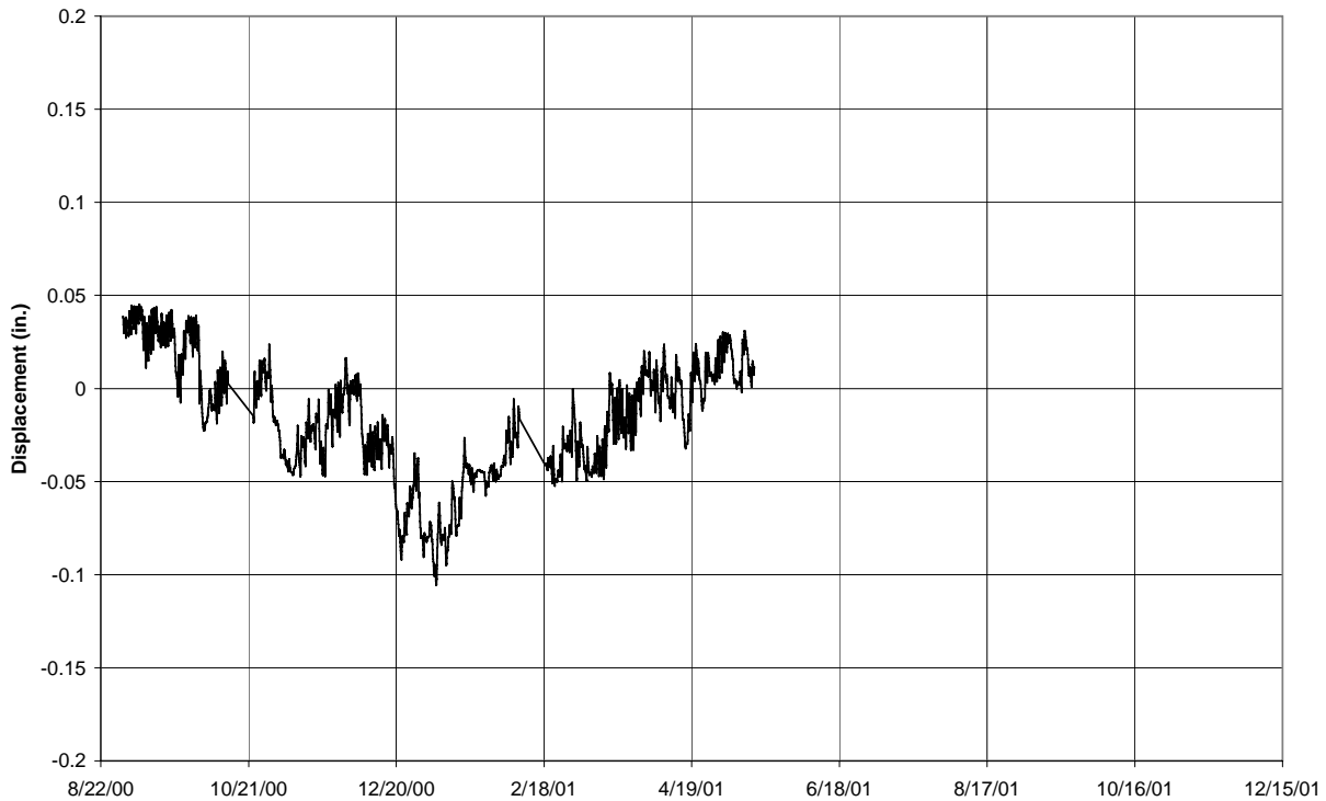
Figure 4.9. Average east abutment displacement
