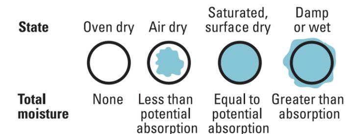
**Figure 2. Saturated, surface dry (SSD) is typically the preferable aggregate moisture state.**
