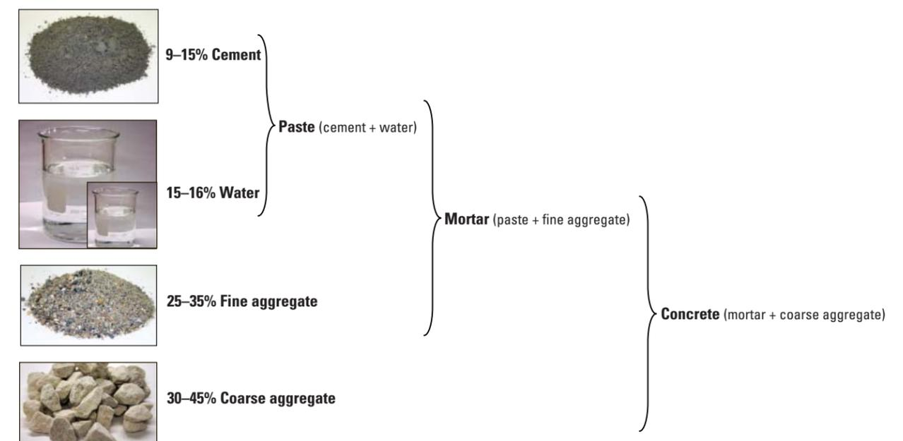
**Figure 1. Concrete is basically a mixture of cement, water/air, and aggregates (percentages are by volume).**
