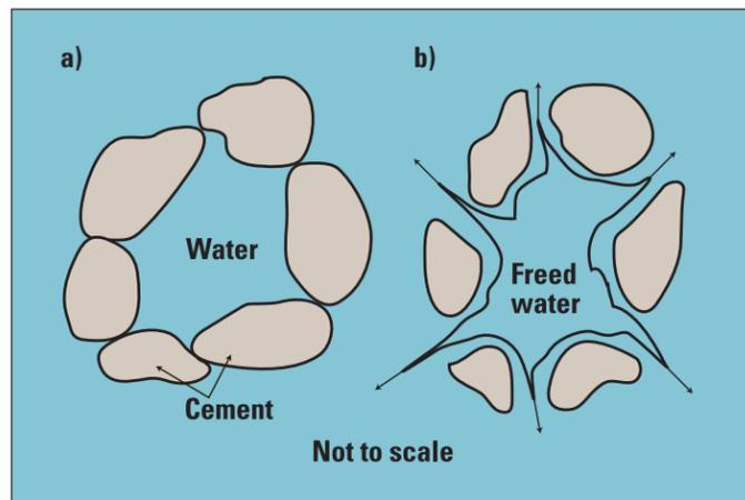
**Figure 3. One mechanism by which water reducers work is dispersion. (a) Charged cement particles cling together, trapping water. (b) Water reducers separate cement grains, releasing the water and making it available for hydration.**
