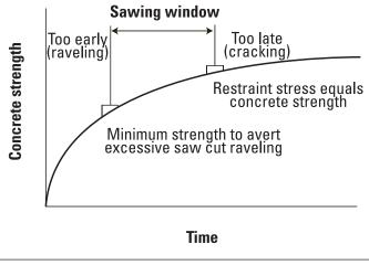
Figure 2. Sawing window
