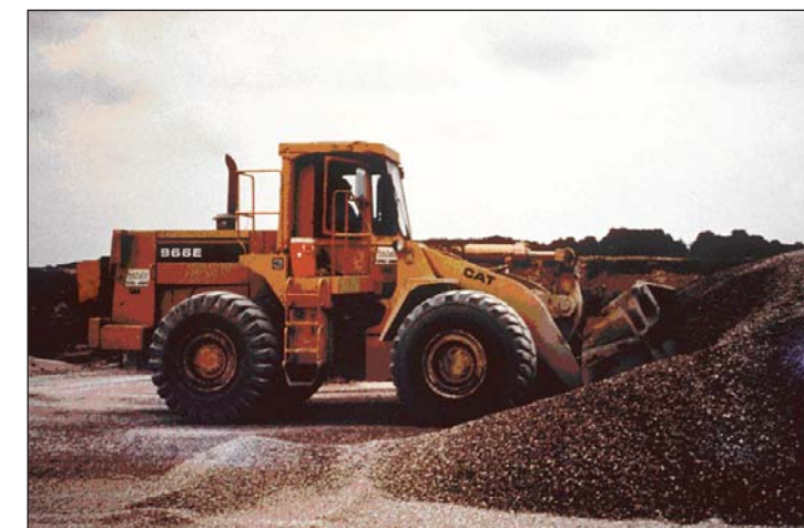
Figure 1. Good stockpile management is important for minimizing aggregate segregation (photo by American Concrete Pavement Association).
