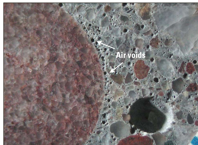
Figure 4-31. A typical example of air voids clustered around an aggregate particle
