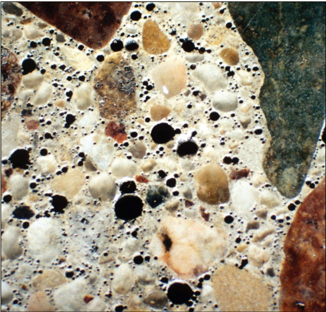
Figure 3-15. Entrained air bubbles in concrete (PCA)
