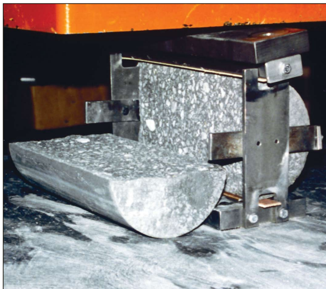
Figure 5-7. Splitting tensile strength (PCA)
