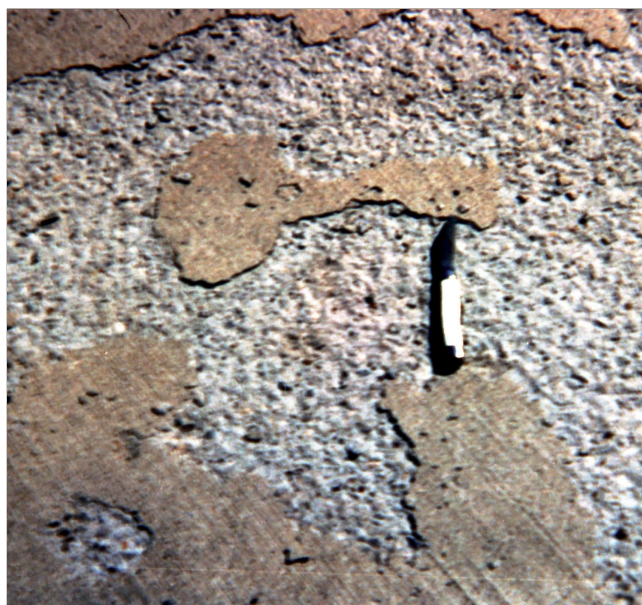
Figure 5-15. Scaled concrete surface resulting from lack of air entrainment, use of deicers, and poor finishing and curing practices (PCA)
