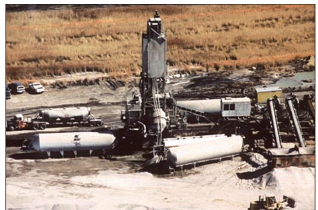
Figure 8-1. Portable concrete plant (ACPA)
