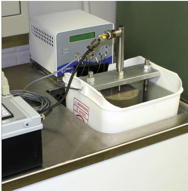
Figure 5-13. Measuring the coefficient of thermal expansion
