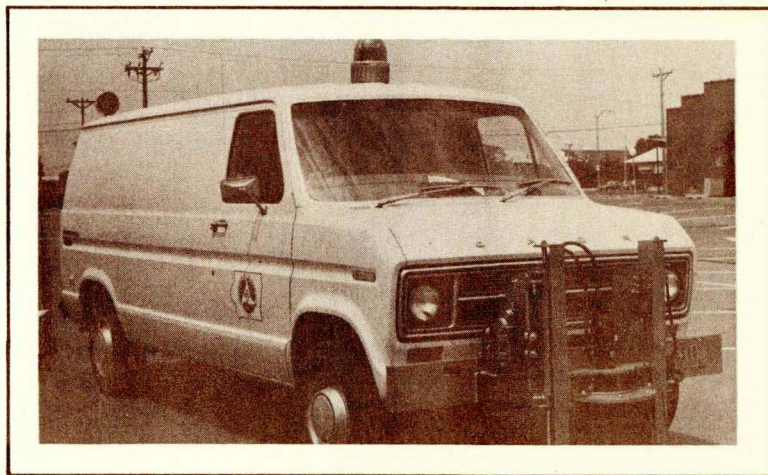
Pavement deflections are measured with a "road rater."
