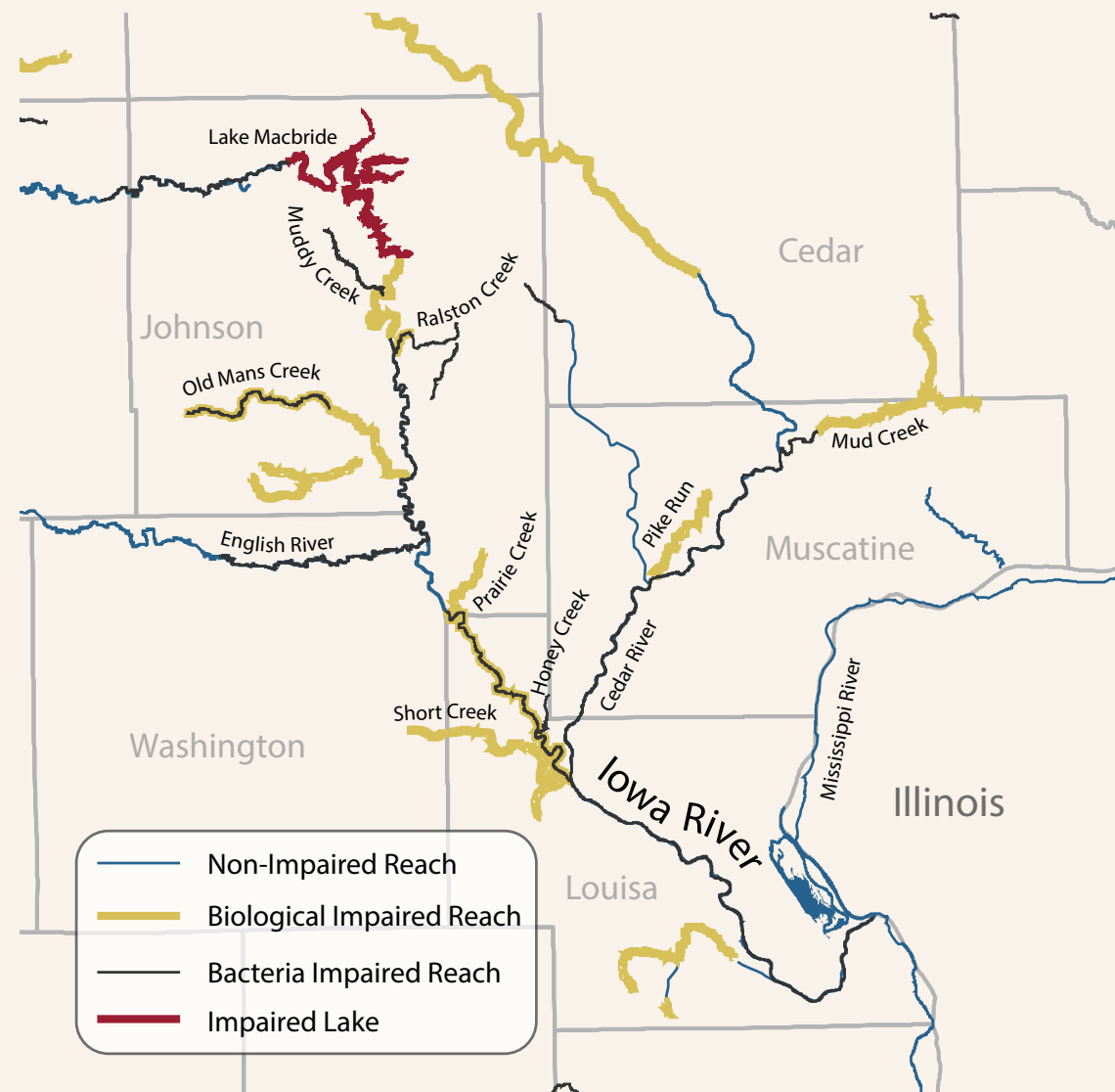
Figure 7 A majority of the water trail is listed on Iowa's 303d List, as well as many tributaries draining into the water trail.
