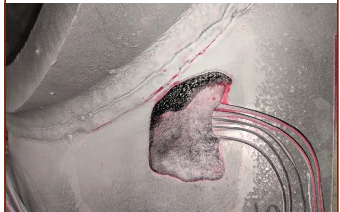
Specimen B-1, with 54% opening ratio hand hole, showed few indications with dye penetrant test after 1,000,000 cycles at 8 ksi
