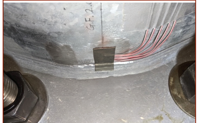
Specimen B-1, with 54% opening ratio hand hole, showed few indications with dye penetrant test after 1,000,000 cycles at 8 ksi
