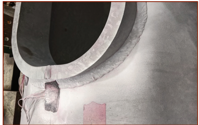
Specimen A-1, with 46% opening ratio hand hole, showed no indications with dye penetrant test after 1,000,000 cycles at 8 ksi
