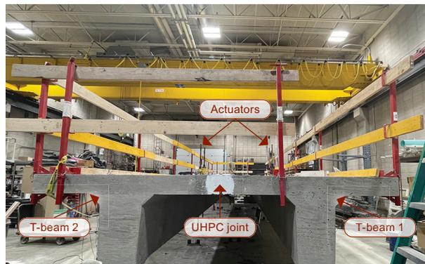
*Full-scale T-beam specimen with longitudinal UHPC joint in Iowa State University's Structural Engineering Research Laboratory*
