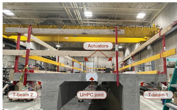
*Full-scale T-beam specimen with longitudinal UHPC joint in Iowa State University's Structural Engineering Research Laboratory*
