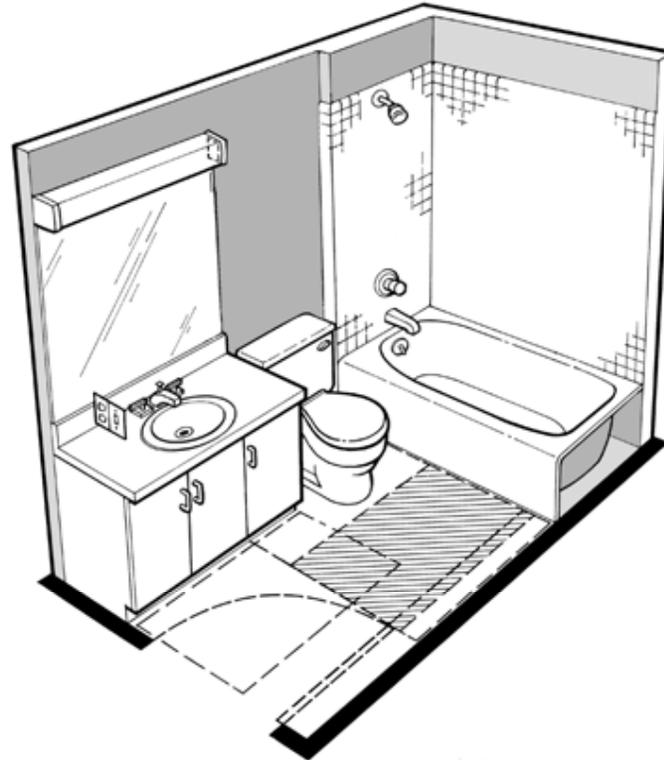
**This illustration shows a conventional in-line bathroom design that would comply with Specification “A”. A distinguishing feature of a Specification “A” bathroom is that a toilet (or lavatory) is permitted to be located within the clear floor space adjacent to the bathtub. In this illustration a toilet is allowed to be positioned next to the bathtub, making access to the bathtub limited.**
