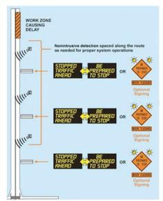
MnDOT Low-cost QWS using multiple detectors and signs A number of intelligent transportation system (ITS) technologies have been developed and are available to provide queue warning. These systems typically use side-fire radar for speed detection and trailer-mounted portable changeable message signs (PCMS) to display the warning message to drivers.
