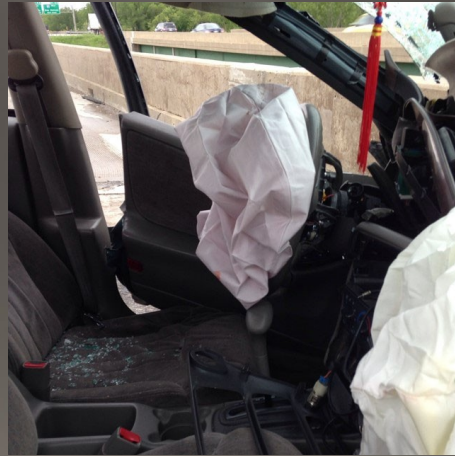
No seat belt (tight against b-pillar)
