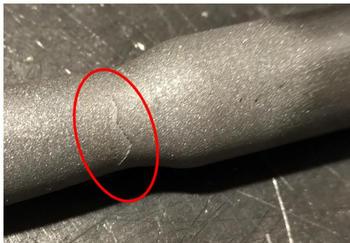
Figure 30. Substrate material flaking off from itself. There is no coating on this specimen
