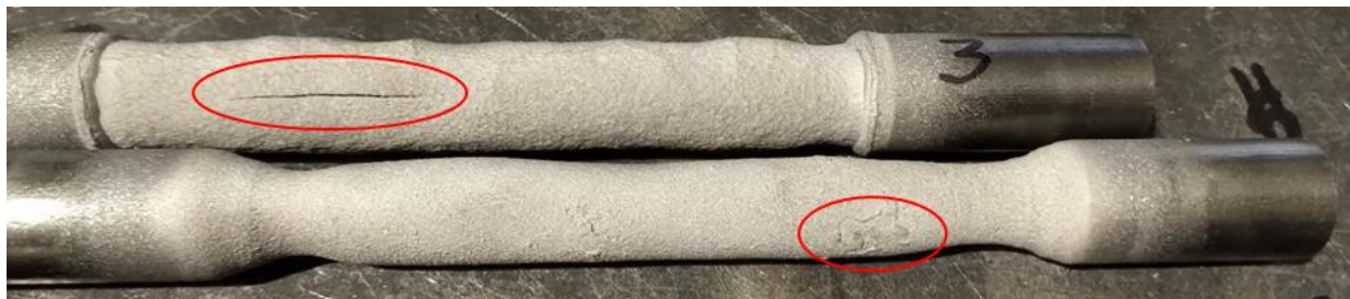
Figure 29. Corroded specimens after coating with Inconel: the upper specimen developed a crack in the deposit as the specimen cooled down; the lower specimen showed “blistering”
