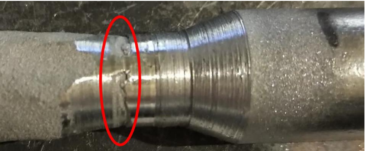
Figure 32. Corroded specimen after attempts to machine down to sound material: more substrate material would “flake” off
