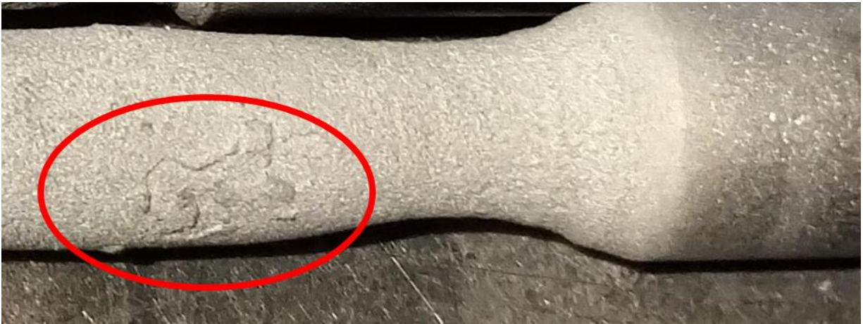
Figure 31. Closeup of “blistering” in Inconel coating on corroded coupon
