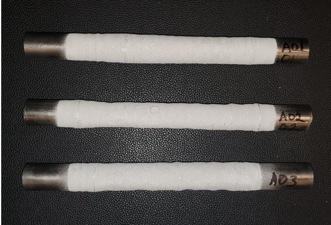
Figure 16. Corroded samples with the mass lost due to corrosion repaired using cold spray coating
