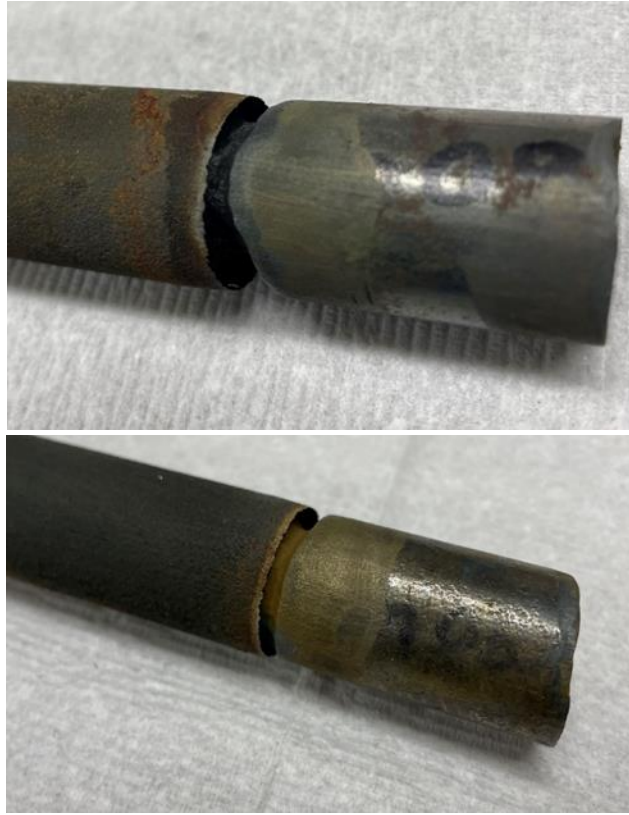
Figure 21. Closeup of corrosion on Inconel bars after 7-days (top) and 14-days (bottom)
