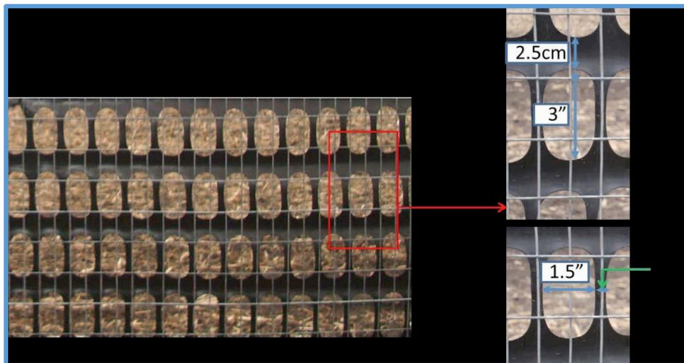
Figure 7. Overlapping wire and plastic meshes to attain prescribed fence porosity at the US-20 test site (Constantinescu and Muste, 2015).
