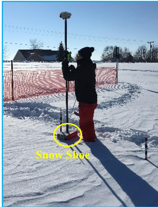
Figure 31. RTK survey conducted at the marker poles located at Shueyville site. The “snow shoe” consists of a  $35 \times 20 \times 9.5 \text{ cm}$  ( $14 \times 8 \times 4 \text{ in}$ ) cardboard box.
