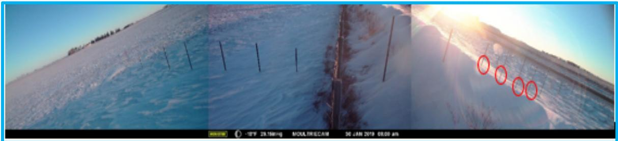
Figure 36 Glare produced at sun on the webcam image at US-20 site (January 30<sup>th</sup>, 2019). The crest of the snow deposit blocks the accurate detection of the marker pole elevations located toward the road (downwind from the fence). The problematic poles are indicated with red circle.
