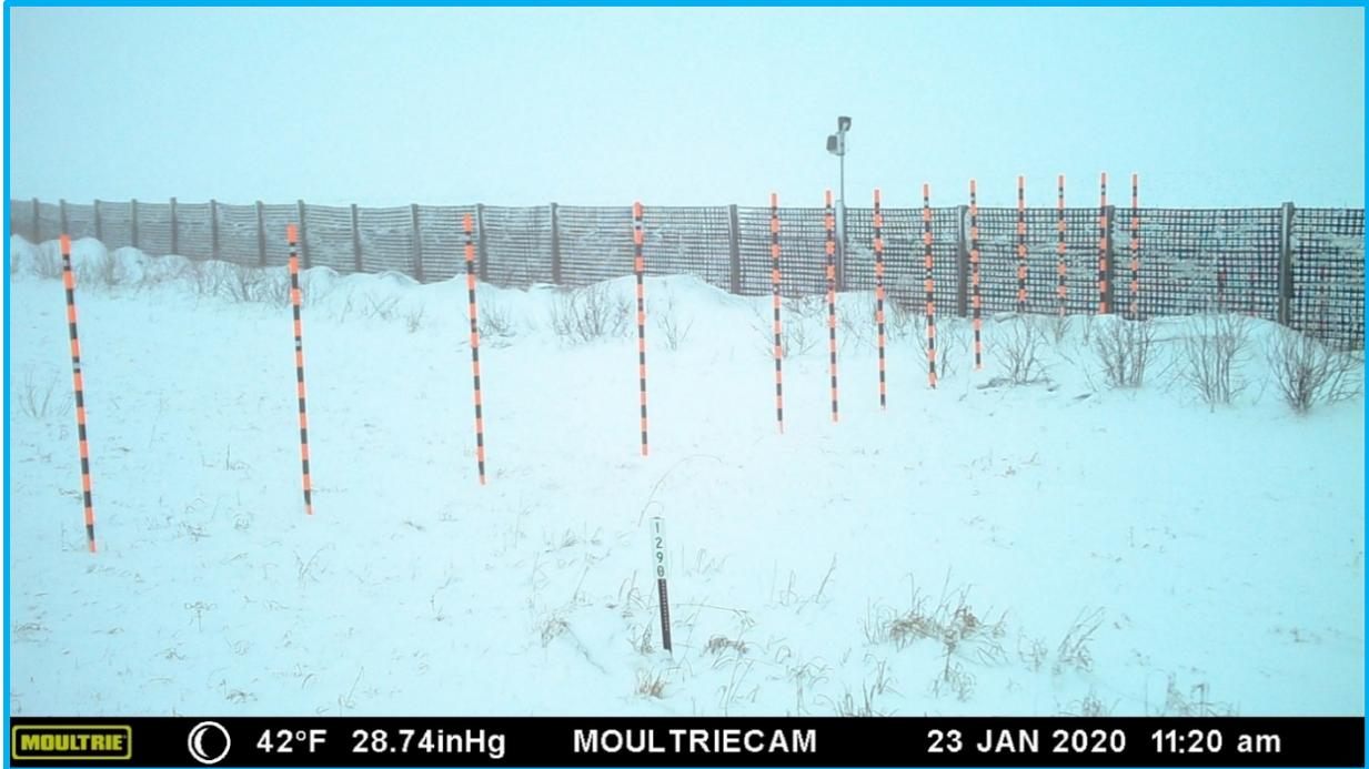
Figure 35. Image taken by redundant webcam on January 23<sup>th</sup>, 2020. Besides providing snow surface elevations while the main webcam is blocked, the strategic positioning of the images acquired with this camera allows to resolve the snow cover elevations for the marker poles located downwind from the snow deposit crest.
