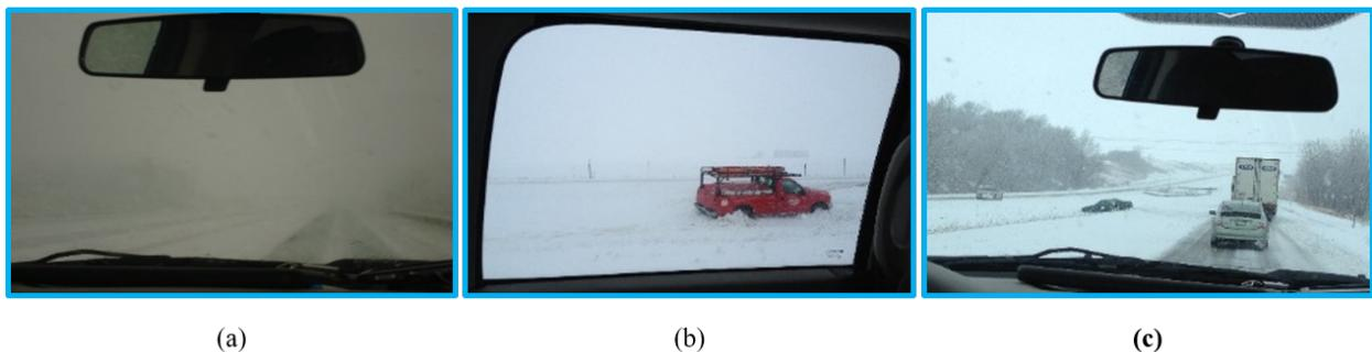
Figure 1 Effects of snow blowing on Iowa's roads: a) reduced visibility; b) accidents, c) reduction of the effective road width (photos: Tsai, 2015, I-35 Hwy, Iowa).
