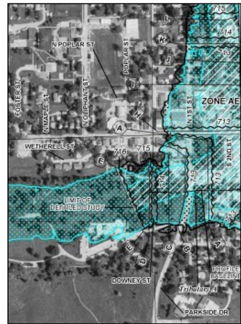
Figure 3-3 Cross sections on a FIRM
