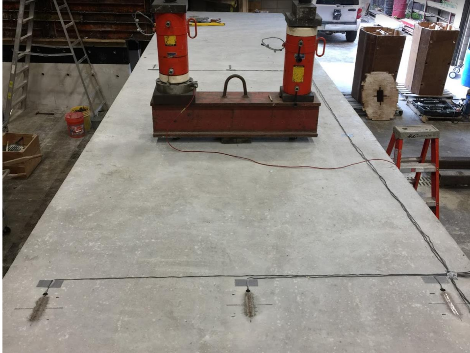
a) Strain gauge arrangement on concrete deck
