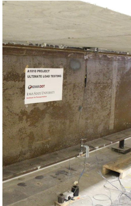
c) LVDT and DCDT at S2 (mid-span)
