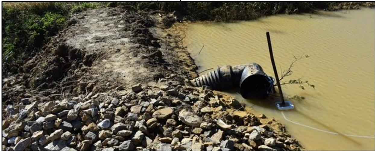
(b) Sample float system at discharge
