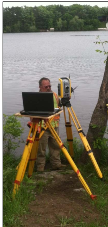
Total Station Collecting Positional Data
