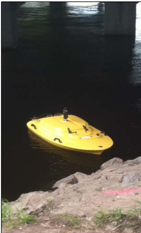
Z-Boat with the GNSS Antenna Replaced with a Reflective Prism
