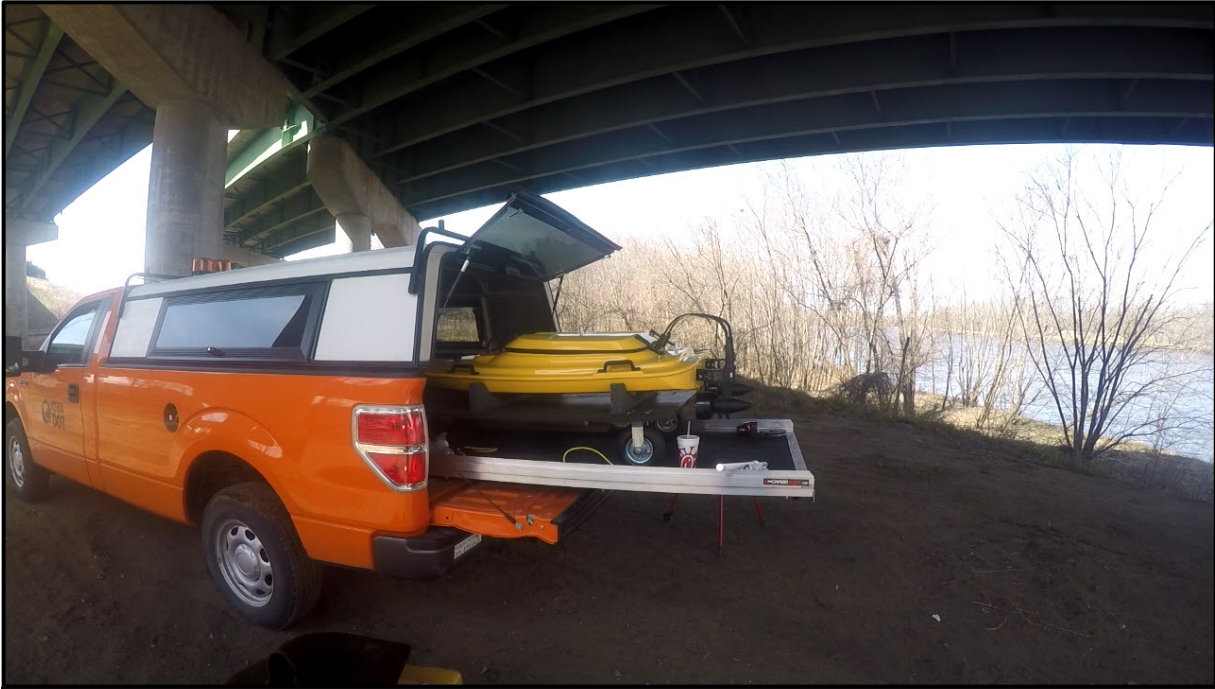
Iowa DOT vehicle fitted with locking topper and roll-out storage platform.
