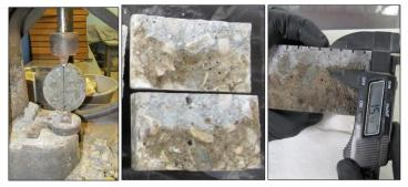
(c) Splitting tested samples and determining chloride penetration depth after 15 minutes of spraying with 0.1 M of silver nitrate
