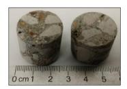
Figure 3.8. Concrete plugs used for MIP analysis
