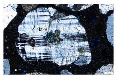
Figure 4.20. Thin-section micrograph highlighting a fine aggregate grain
