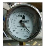
(a) Air meter reading zero with full water during calibration
