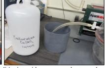
(c) Sample conditioning with vacuum and saturated  $Ca(OH)_2$  solution
