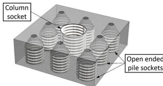
*Precast pile cap with preformed sockets*
