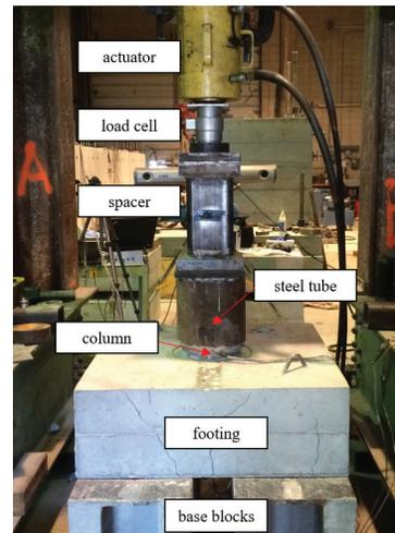
*Test setup for socket connection tests*
