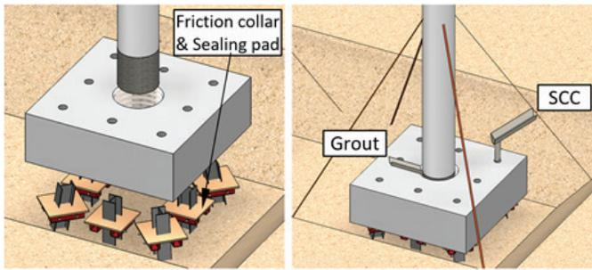
*Construction of column/footing/pile system*
