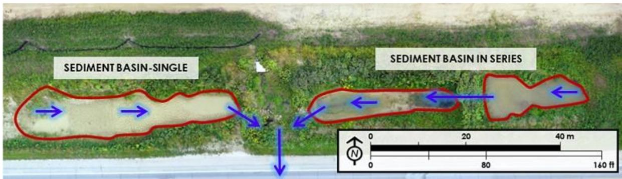
**Figure 6.6. Modified temporary sediment control basin design**
