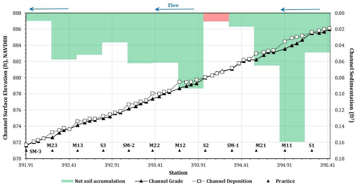
**Figure 4.11. Silt fence ditch check channel grade profile**
