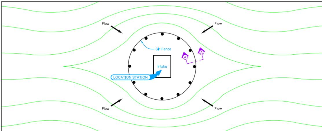
PLAN FOR SILT FENCE AT INTAKE (TYPE 2) <sup>12</sup>
