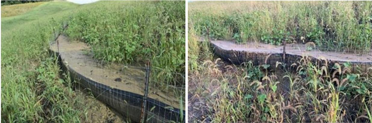
(a) Full sedimentation, no deflection (9/5/2019) (b) Overtopping due to full height sedimentation (9/24/2019)
