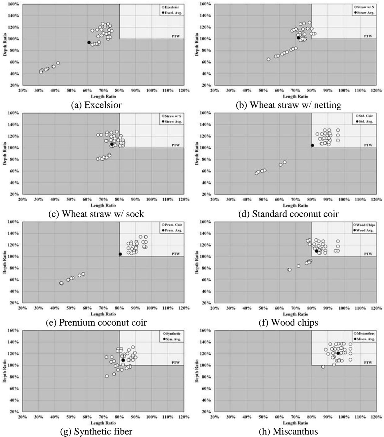
**Figure 7.3. Comparison of depth ratio to length ratio**
