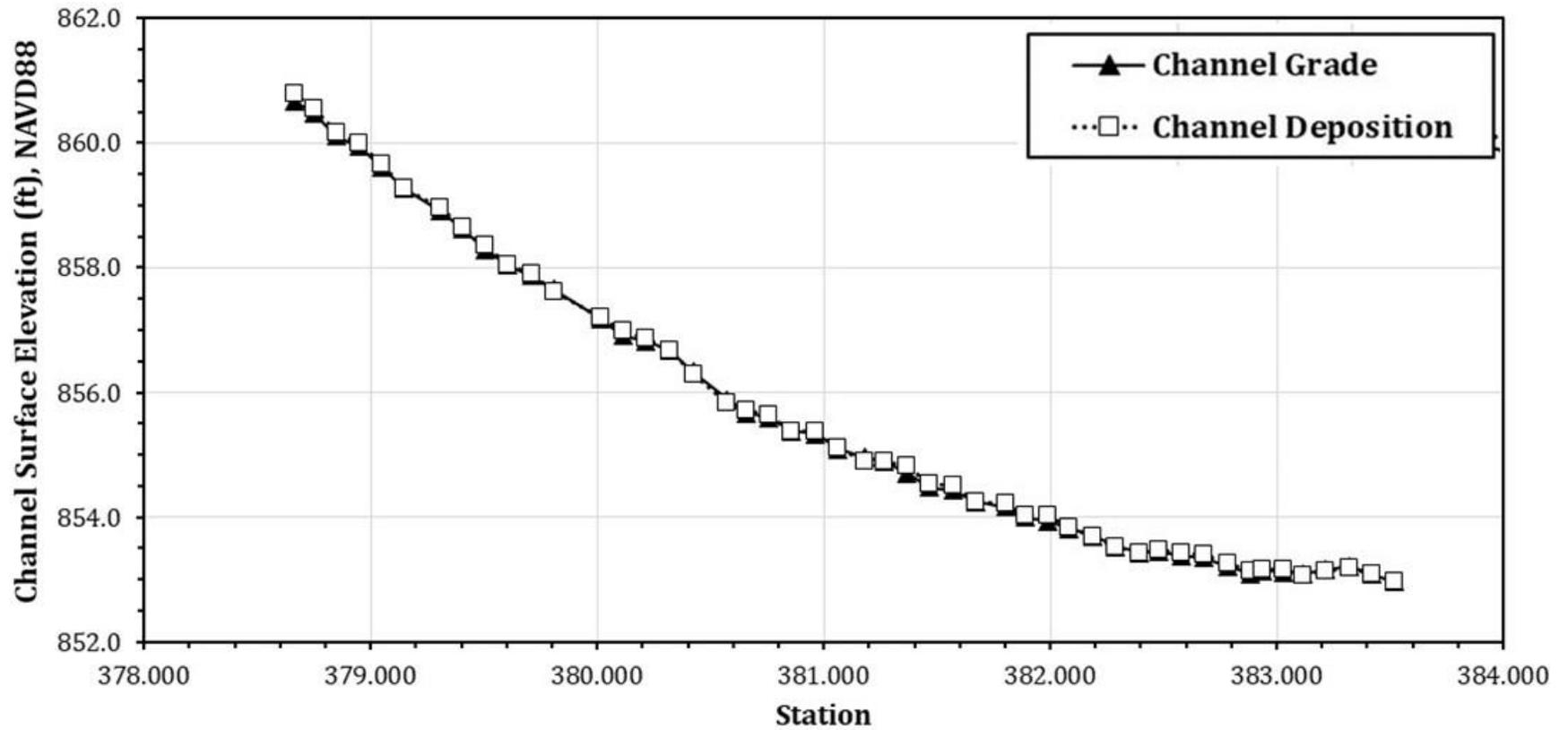
Figure F.10. Excelsior wattle ditch check channel profile
