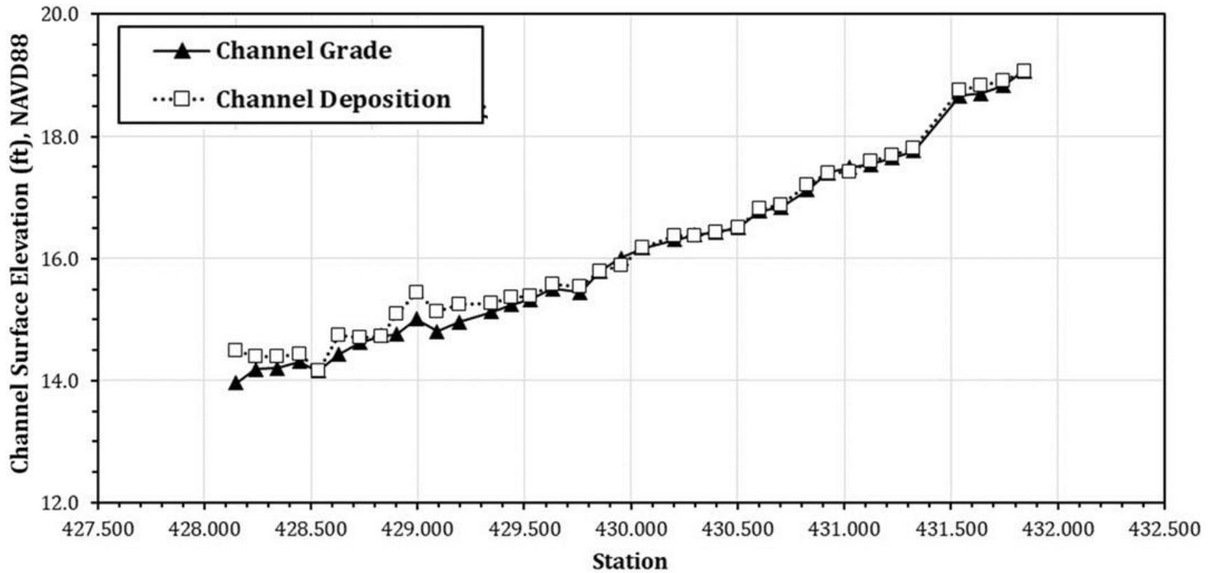
Figure F.19. Straw wattle ditch check channel profile
