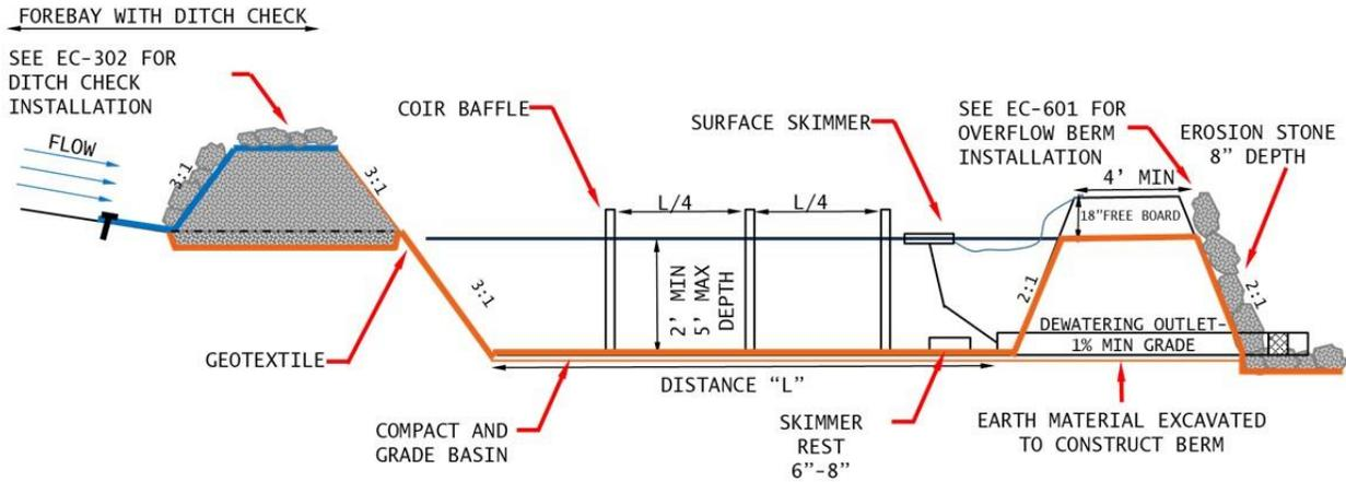
NOTE: SKIMMER AND OUTLET PIPE TO BE DESIGNED TO MATCH BASIN VOLUME AND DEWATERING
