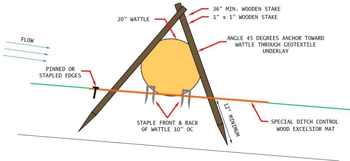
**Figure B.5. Wattle ditch protection - modified detail 1**
