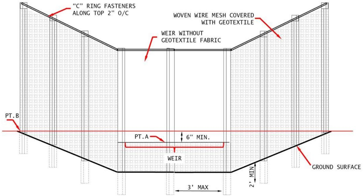
**Figure B.4. Silt fence ditch check weir**
