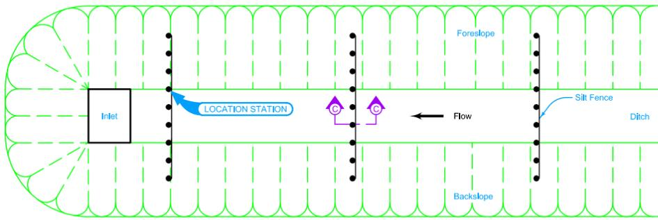
PLAN FOR SILT FENCE DITCH CHECK AT INLET (TYPE 3) <sup>12</sup>
