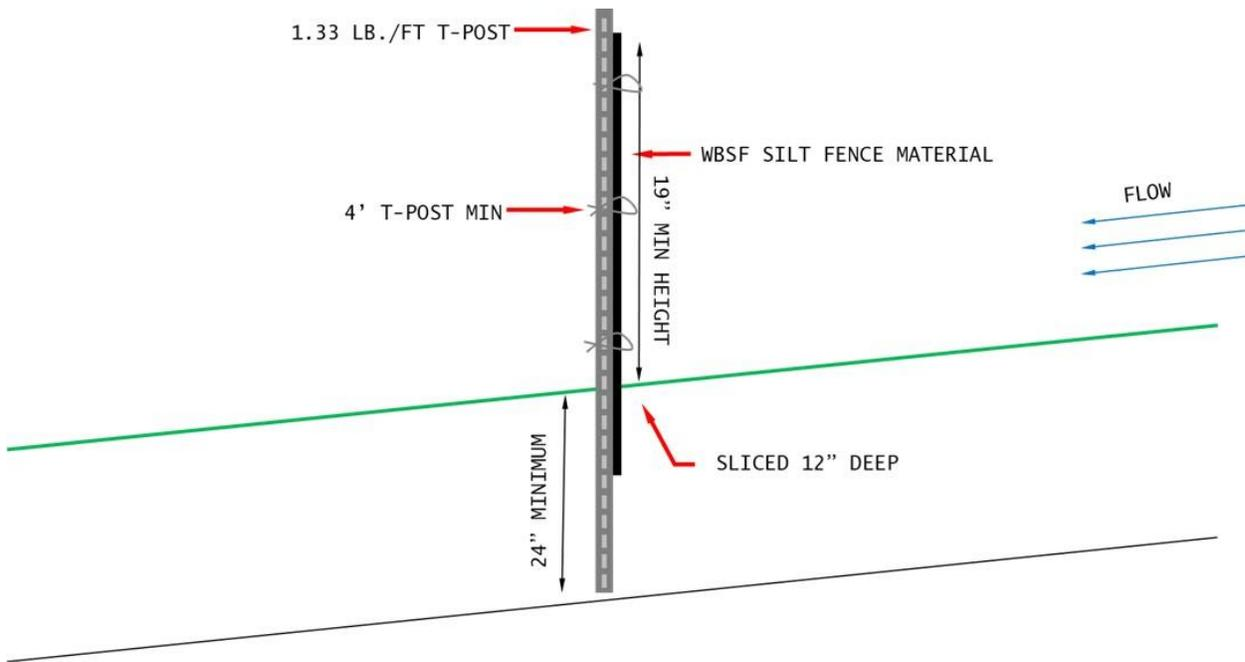
**Figure B.8. Silt fence perimeter control – Standard-M**
