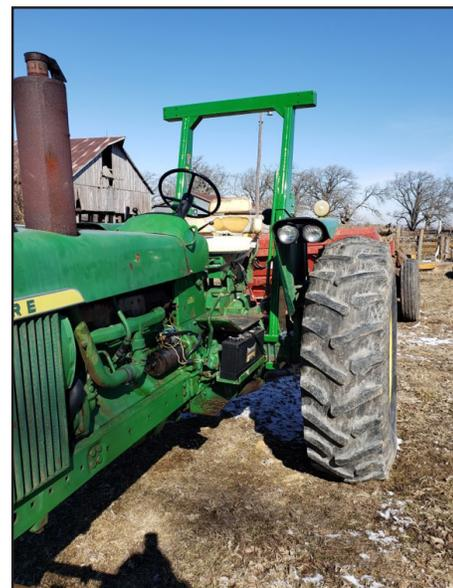
A 1968 John Deere 4020 tractor in Scott County, Iowa after ROPS installation.
