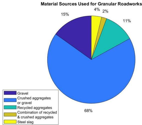
**Figure A-1. Aggregate materials used for granular roadworks**
