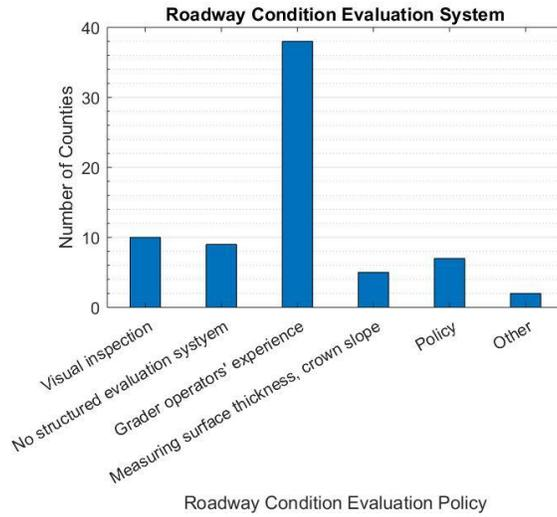
**Figure A-9. Roadway condition evaluation system**
