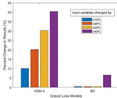
**Figure 4-18. Sensitivity analysis of HDM-4 and BR models**
