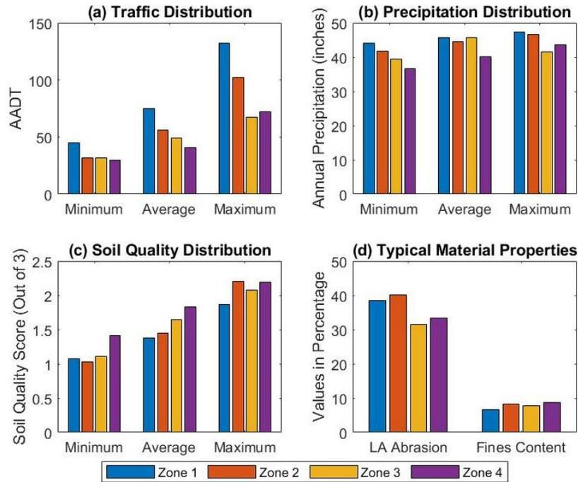
**Figure 4-5. Characteristics of Iowa zones: (a) daily traffic distribution, (b) annual precipitation distribution, (c) soil quality distribution, and (d) typical material properties**
