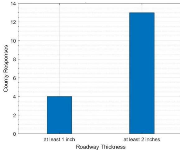
**Figure 4-16. Minimum acceptable roadway thickness**
