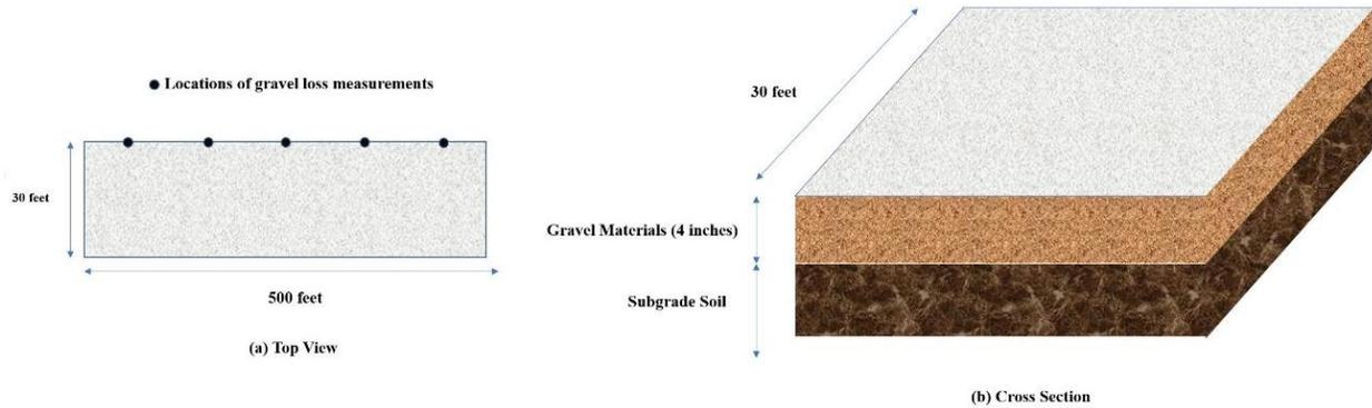
**Figure 4-6. Roadway test site (a) top view and (b) cross section**
