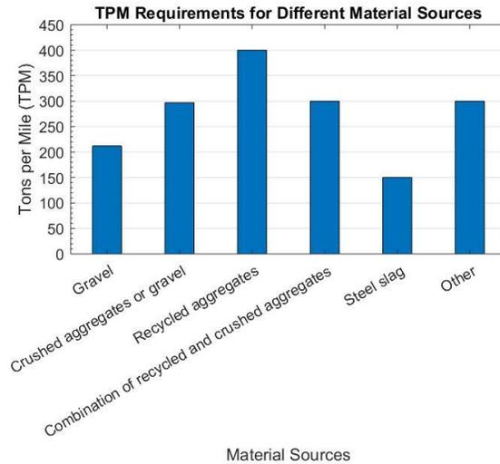
**Figure A-2. Ton per mile aggregate requirements**
