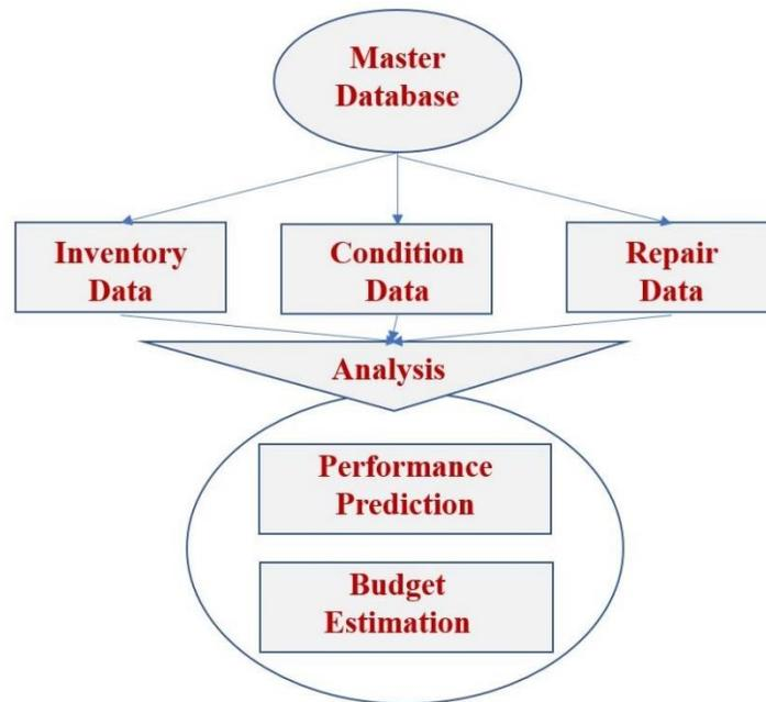
**Figure 2-3. Components of granular roadway asset management system**
