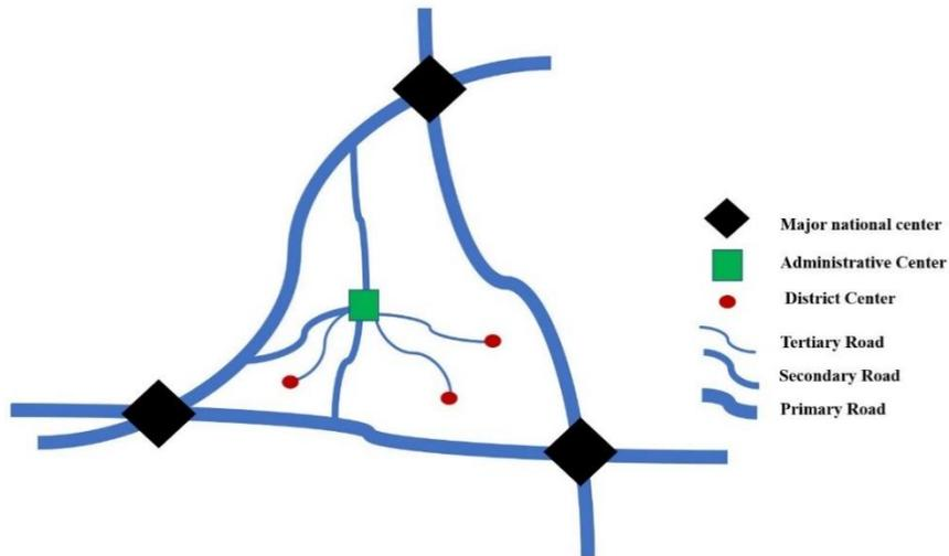
**Figure 2-1. Functional hierarchy of roadway network**
