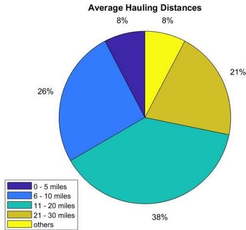
Figure A-4. Hauling distances from aggregate sources
