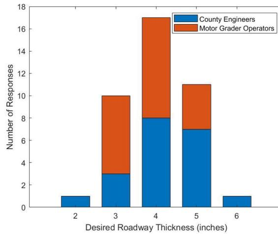
**Figure 4-11. Desired minimum thickness of granular roads for excellent condition**
