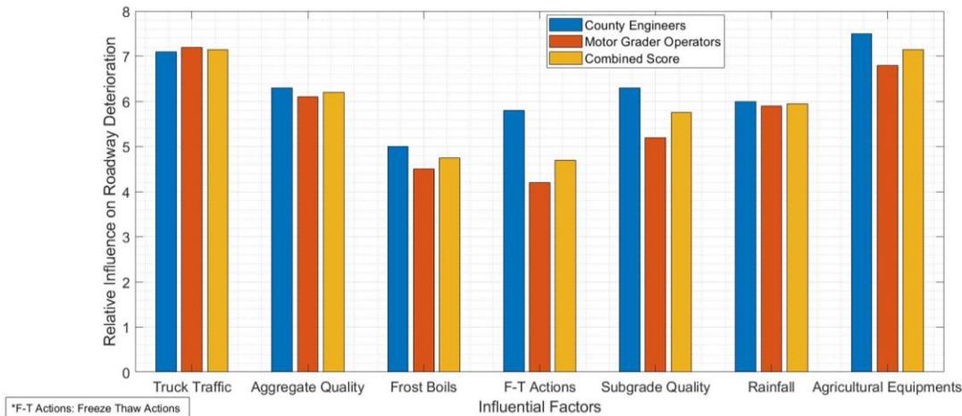
**Figure 4-15. Ranking of granular roadway deterioration influential factors**
