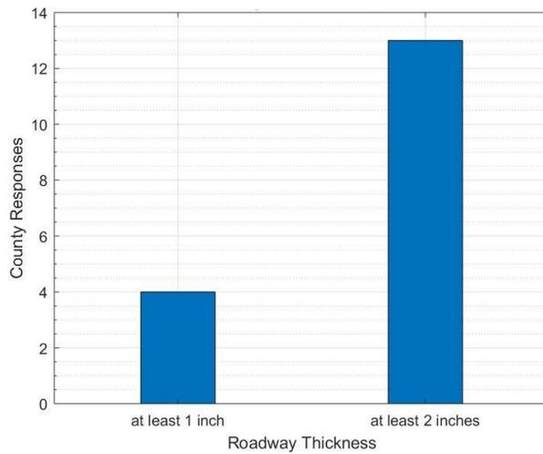
**Figure 4-13. Minimum roadway thickness to trigger maintenance activities**
