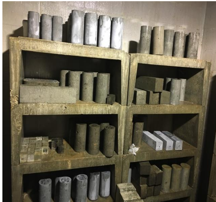
Figure 4.4 Samples placed in the moist curing room after 4 days of steam curing
