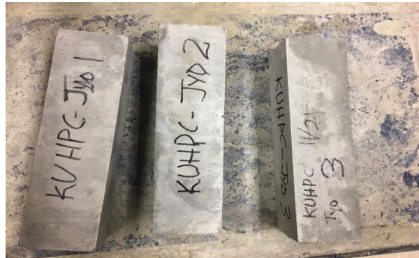
Figure 4.15 Beam shrinkage samples
