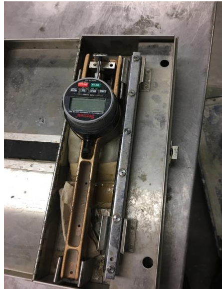
Figure 4.19 Demec gauge with the reference bar
