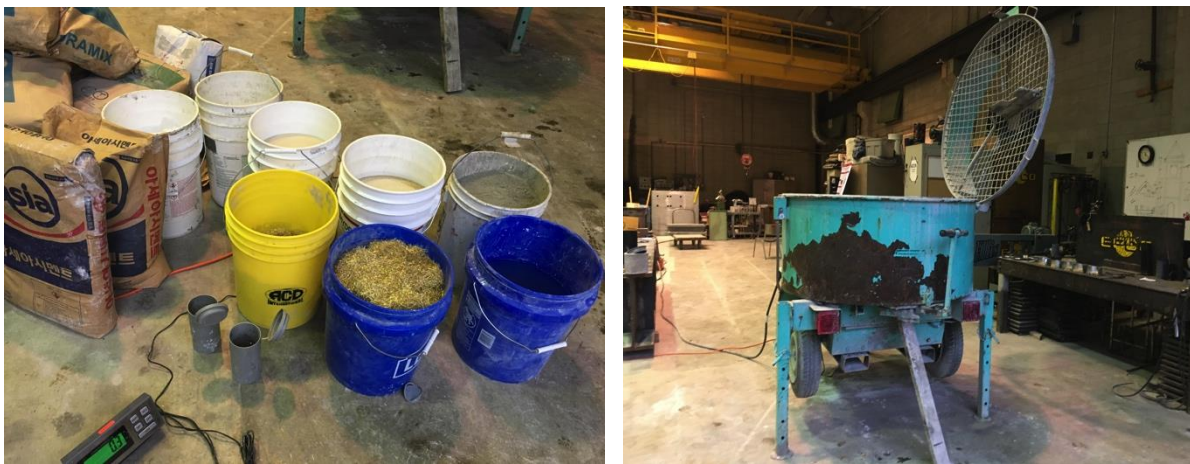
Figure 4.1 Materials ready for mixing (left) and vertical mixer used for mixing K-UHPC (right)
