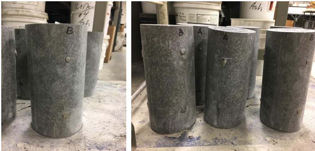
Figure 4.20 Cylindrical samples with Demec discs glued to the surface
