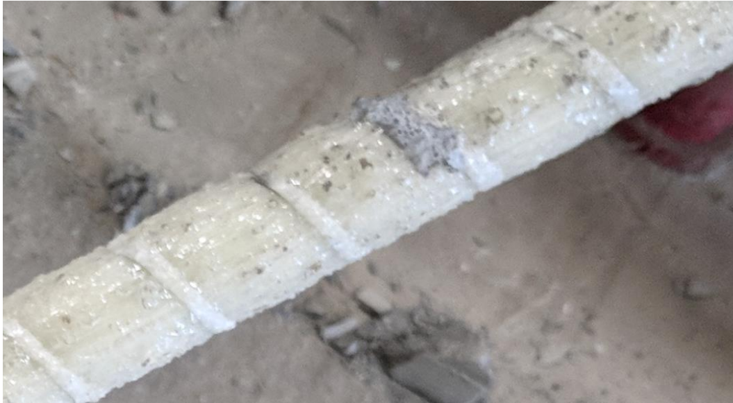
Figure 4.39 Sand/glass fiber GFRP coating
