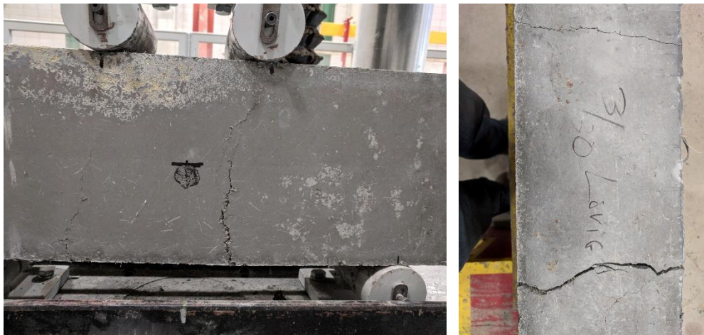
Figure 4.35 K-UHPC cracks at failure
