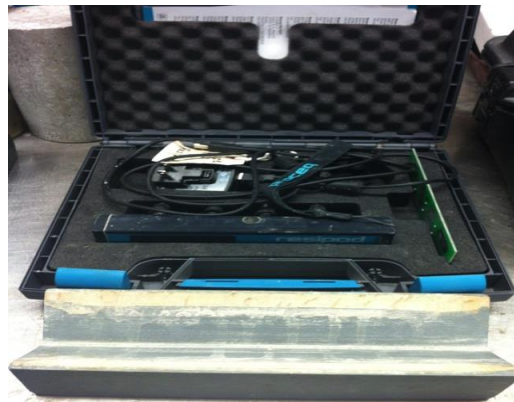
Figure 3.23 Wenner four-electrode device and V-shaped stand
