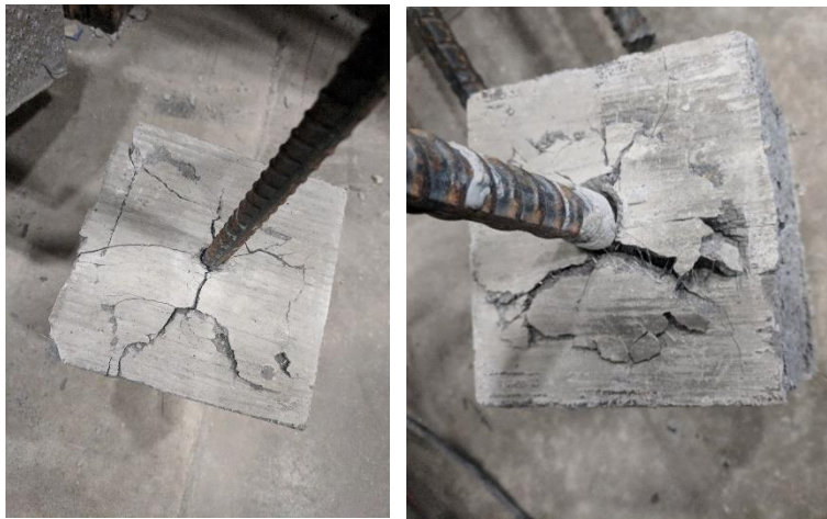
Figure 4.26 UHPC pullout cube slip failure
