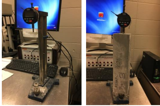
Figures 4.16 Length comparator used to measure shrinkage
