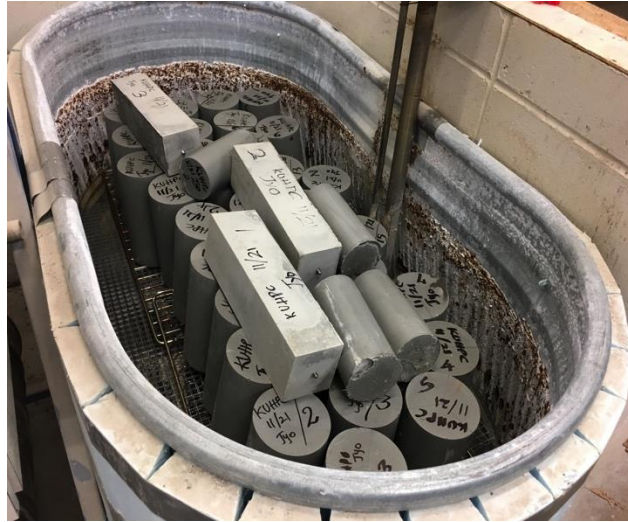
Figure 4.3 Samples placed in steam-curing tank
