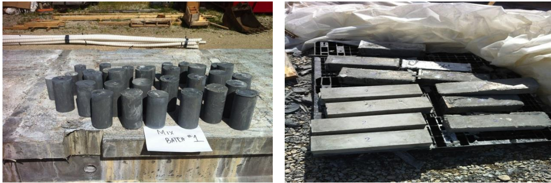
Figures 3.15 Samples after removal from molds and after curing
