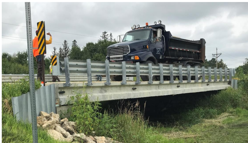
Figure 5.7 Load truck on bridge for LP1
