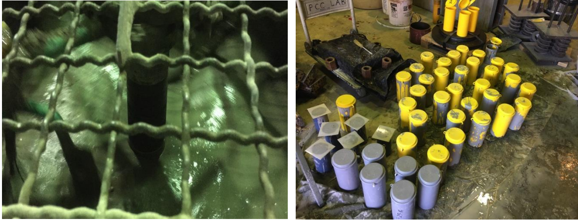
Figure 4.2 K-UHPC while mixing (left) and cylindrical molds after casting (right)
