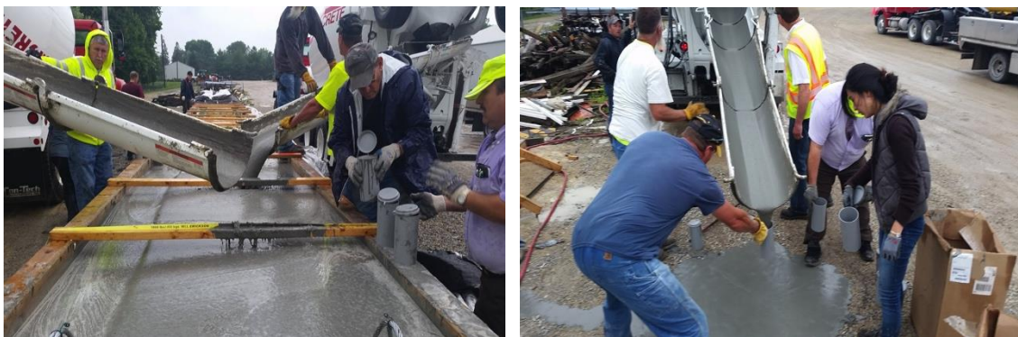
Figures 3.14 Pouring the concrete into the cylindrical molds
