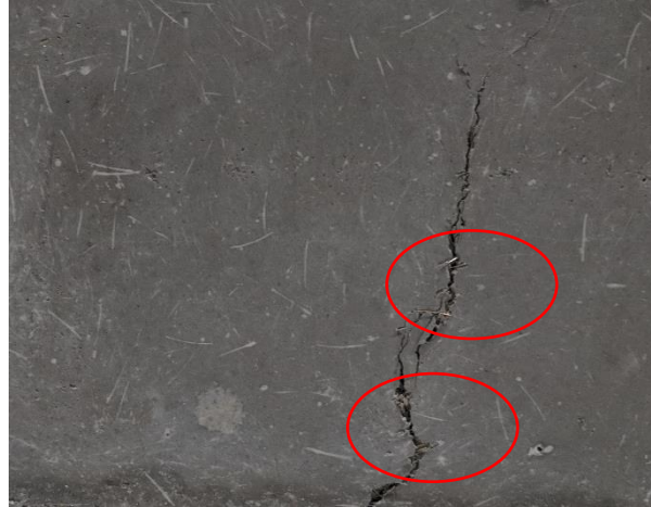
Figure 4.36 Steel fibers reinforcing concrete crack in K-UHPC
