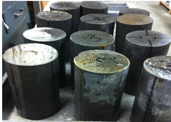
Figure 3.22 Cylindrical samples used for testing with probe lines marked on them
