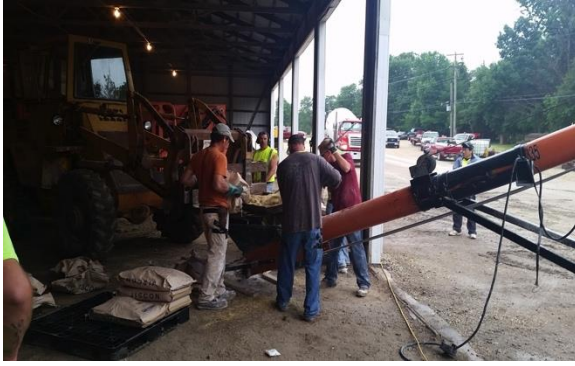
Figure 3.7 Using conveyor for additives (left) and mesh-vibrator for steel fibers (right)
