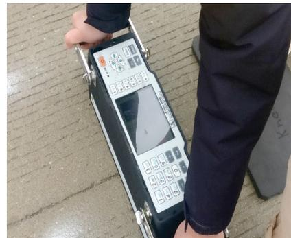
*MIRA ultrasonic shear-wave tomography device being used to collect joint activation data*
