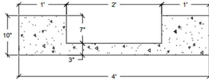
**Figure 24. UHPC-flowability test design proposed cross-section**
