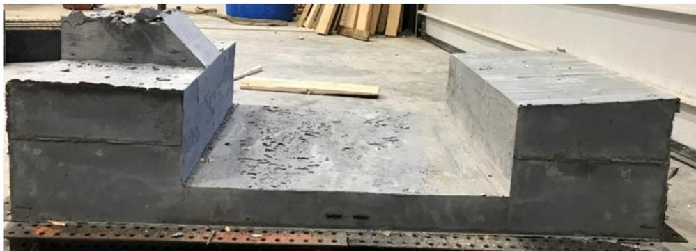
**Figure 32. UHPC flowability test completed**
