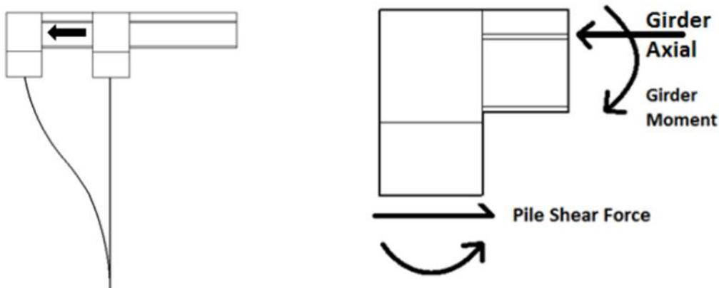
**Figure 54. Structural analysis for thermal expansion of bridge**
