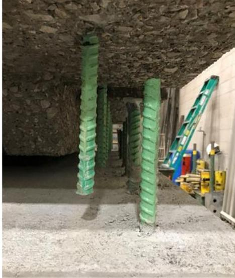
**Figure 44. UHPC joint rear connection bars with adequate clearance**
