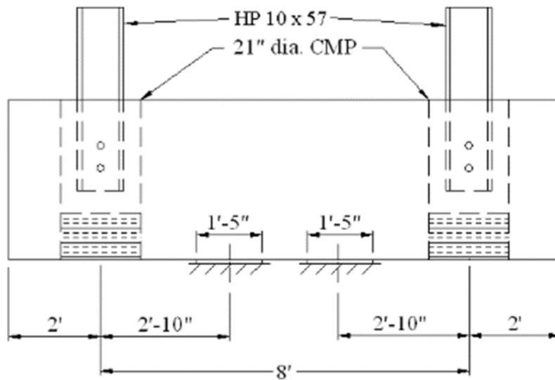
**Figure 3. Double-pile abutment test support details**
