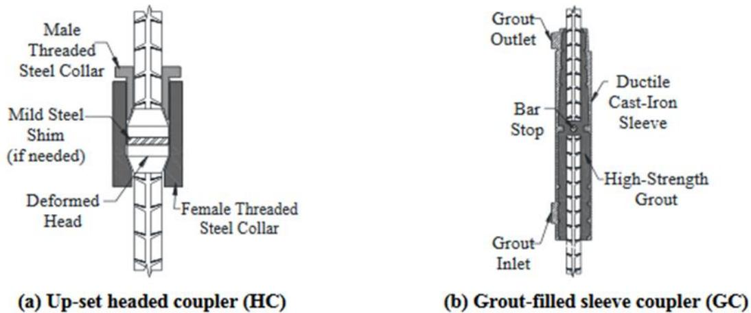
**Figure 5. Mechanical splices used for this investigation**
