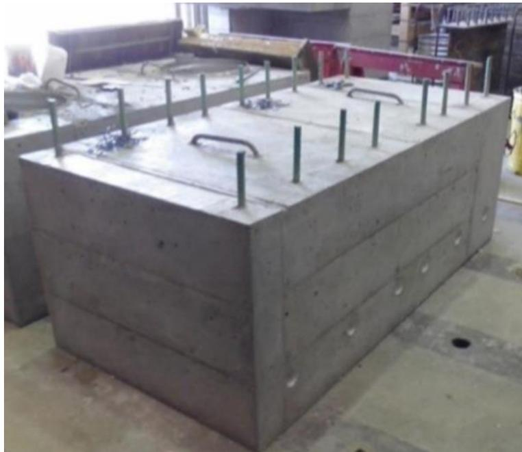
**Figure 12. Grouted reinforcing bar coupler pile cap**
