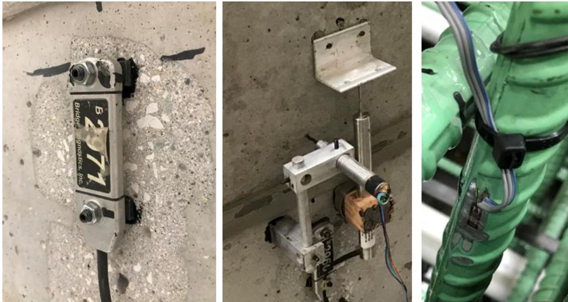
**Figure 57. External strain gauge, left; vertical displacement transducer, horizontal displacement transducer, and external strain gauge, center; and sacrificial strain gauge, right**
