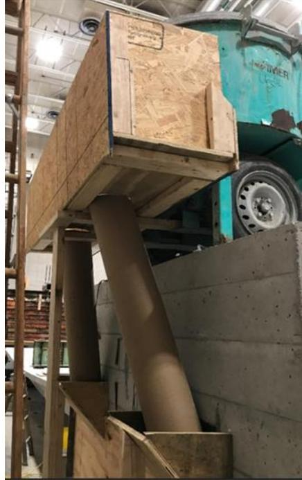
**Figure 48. Spout and chimney system for installation of UHPC material**
