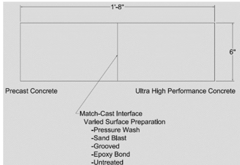
**Figure 8. Simulated MOR test specimen**
