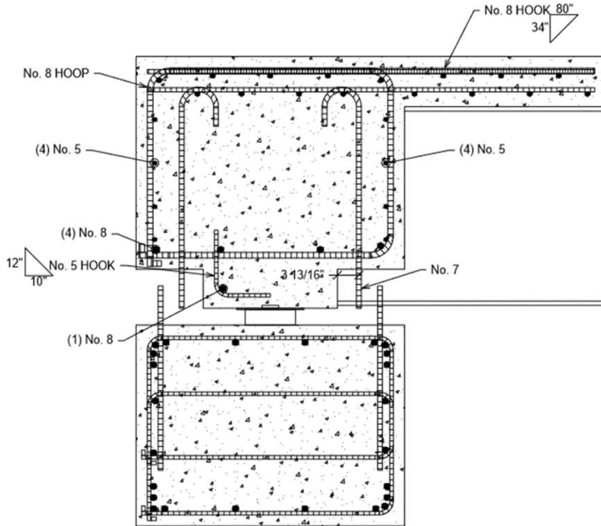
**Figure 21. UHPC joint specimen section view**
