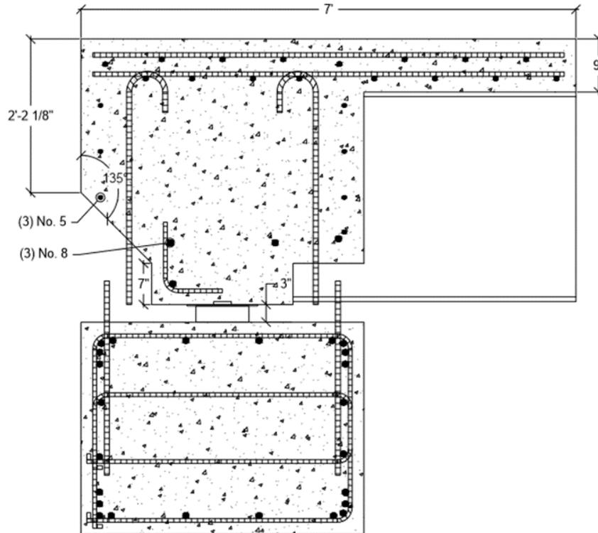
**Figure 20. UHPC joint specimen section through “chimney”**
