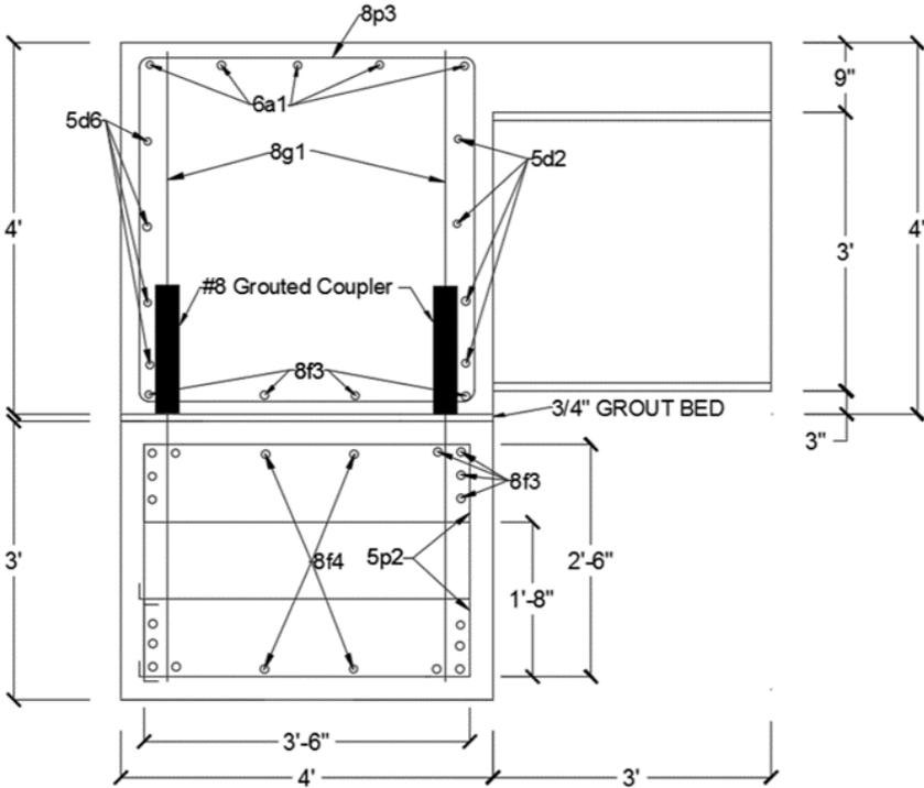
**Figure 9. Grouted reinforcing bar coupler**
