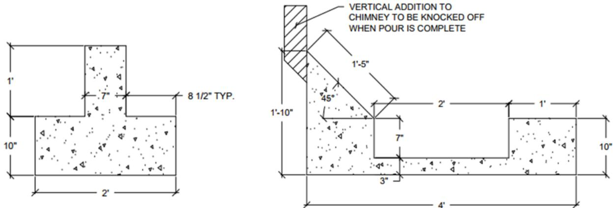
**Figure 26. UHPC-flowability test setup design “chimney” cross-section**
