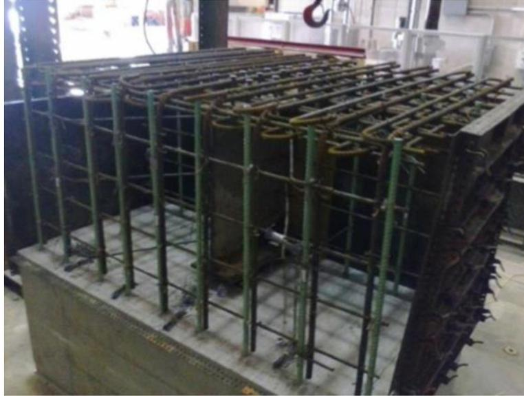
**Figure 11. Cast-in-place specimen reinforcing cage**
