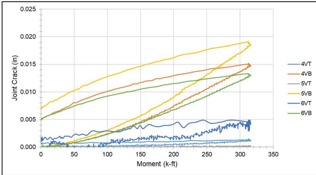
**Figure 58. Crack width versus moment due to horizontal load**
