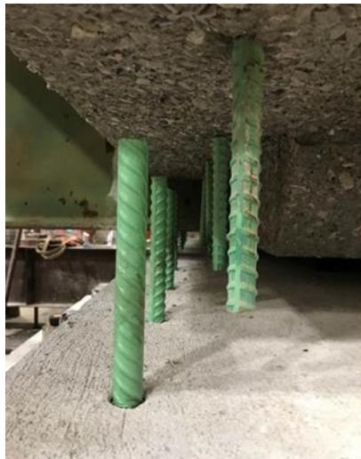
**Figure 45. Front connection bars**
