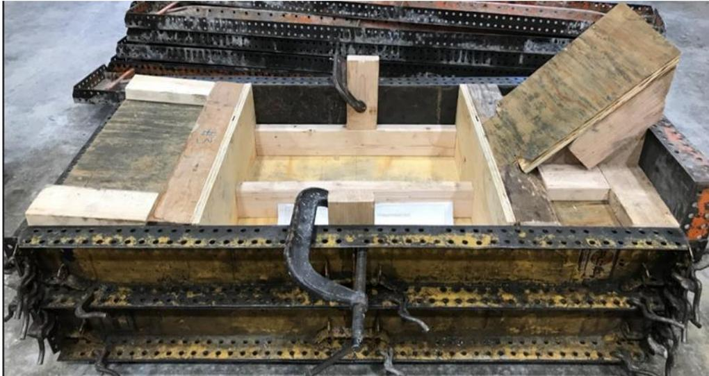
**Figure 31. UHPC flowability test formwork**
