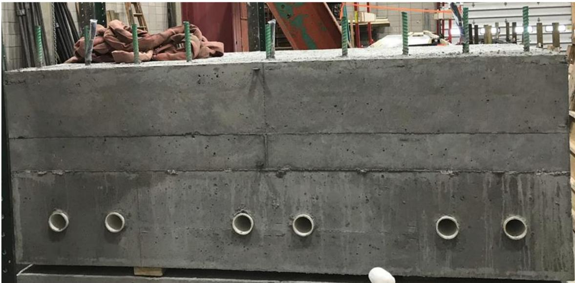
**Figure 30. UHPC joint pile cap completed**
