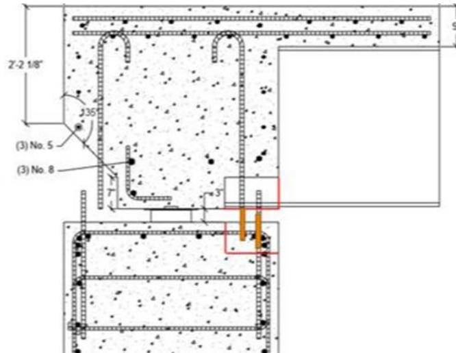
**Figure 63. Proposed revision to UHPC joint connection detail**
