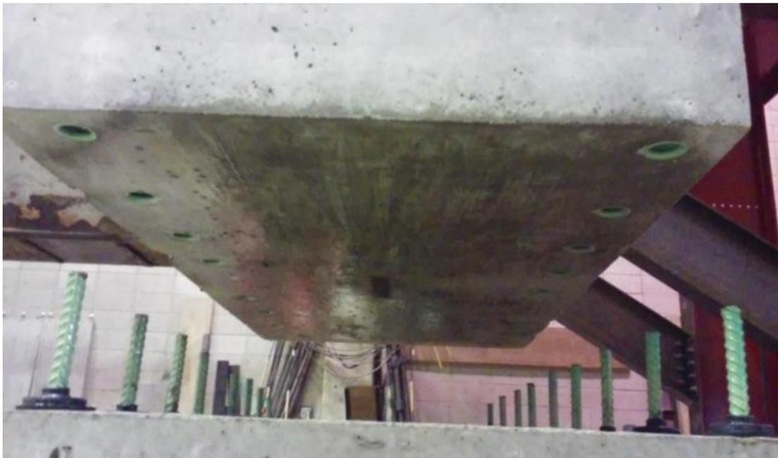
**Figure 14. Grouted reinforcing bar coupler connection placement**
