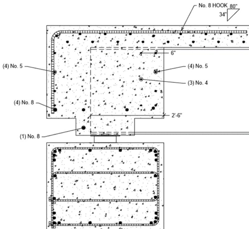
**Figure 22. UHPC joint specimen section view through beam**
