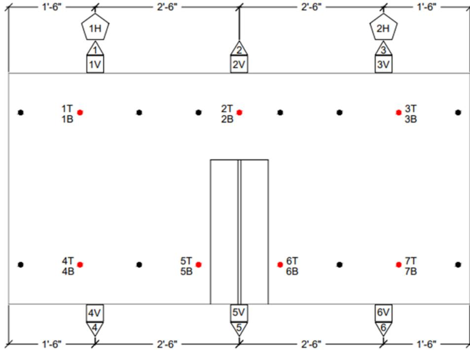
Squares represent vertical displacement transducers; pentagons represent horizontal displacement transducers; triangles represent external strain gauges; and red dots represent locations of sacrificial strain gauges
