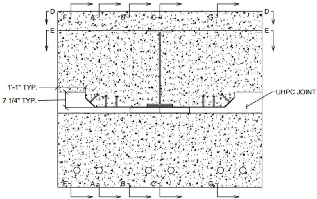
**Figure 23. UHPC joint specimen front view showing “sliding shoes” and pads**
