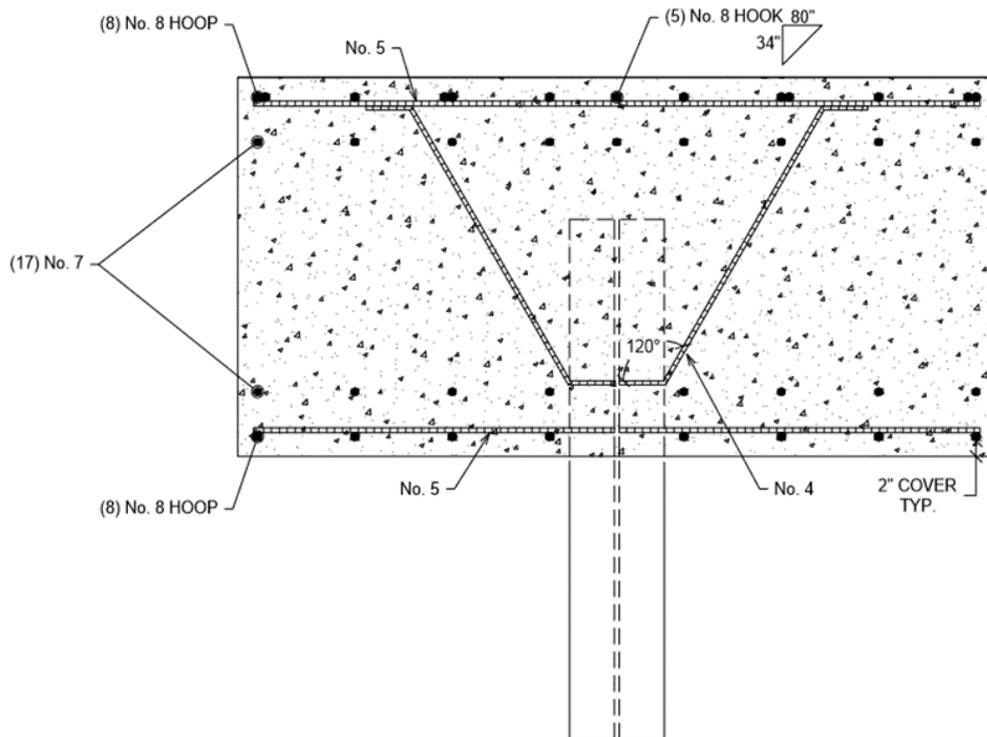
Figure 19. Plan view of UHPC joint specimen showing locations of connection bars
