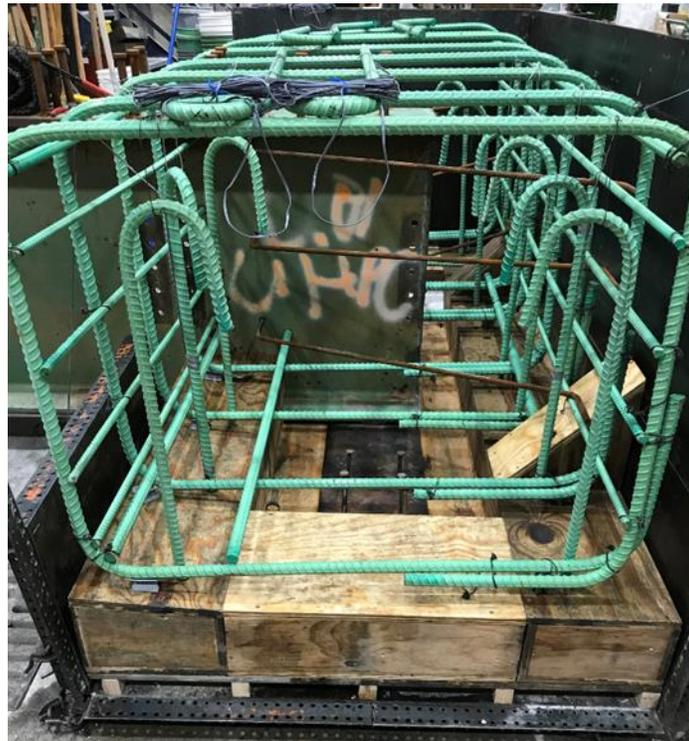
**Figure 36. UHPC integral diaphragm reinforcement cage**
