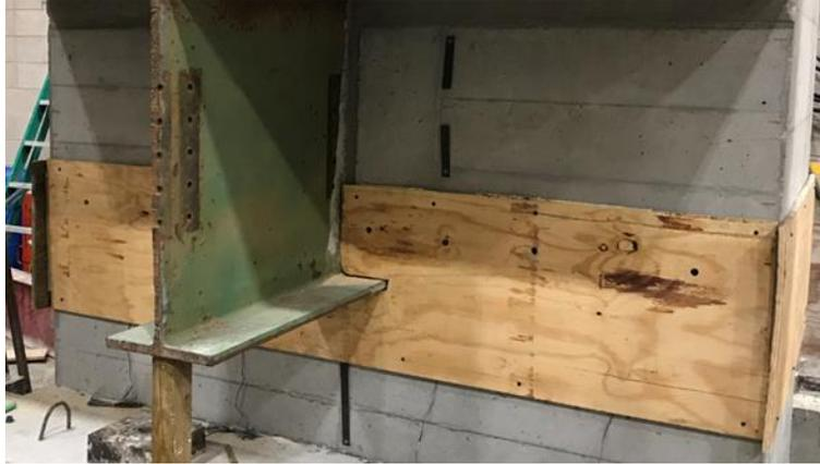
**Figure 46. Front face joint formwork with air ports**
