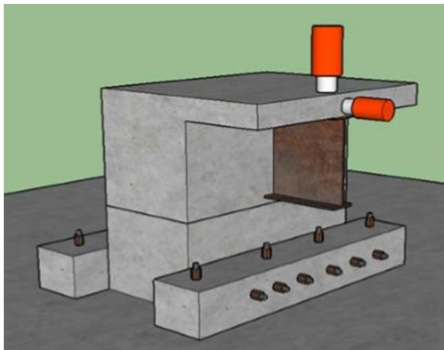
**Figure 18. Laboratory setup for integral abutment specimens**
