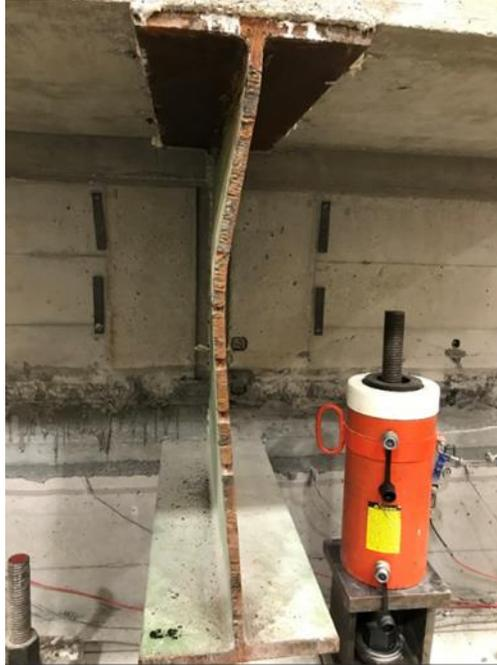
**Figure 59. Beam buckling failure causing end of test**
