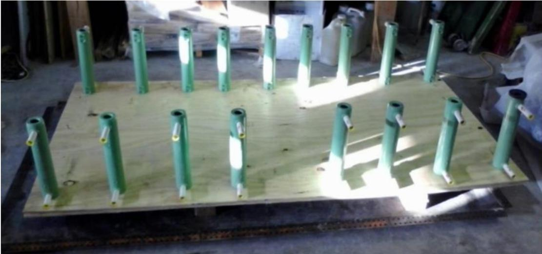
**Figure 13. Grouted reinforcing bar coupler template used for match-casting**
