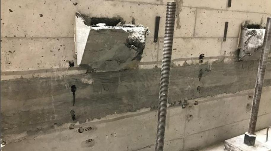
**Figure 61. UHPC joint rear face after testing**
