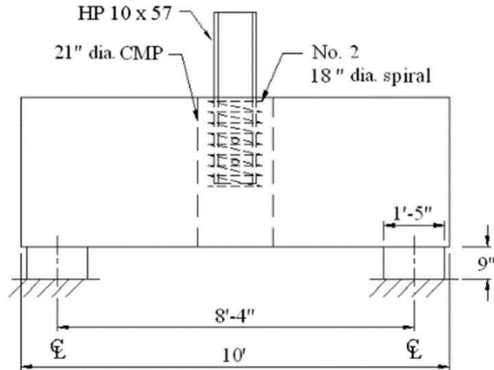
**Figure 2. Single-pile abutment test support details**
