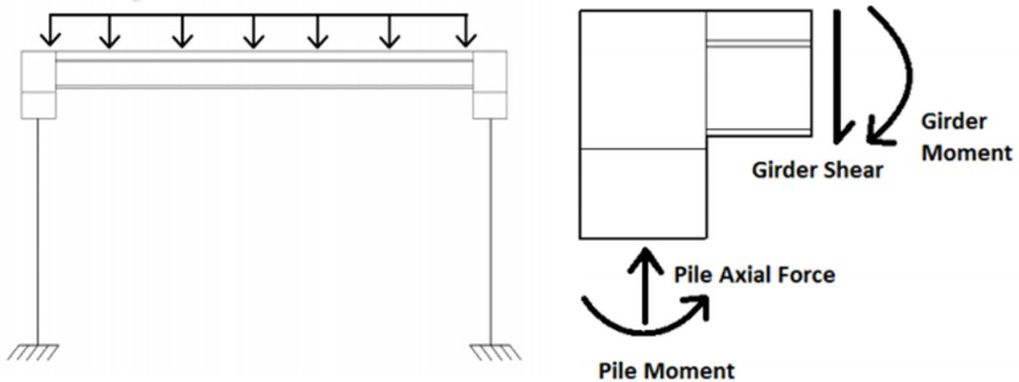
**Figure 55. Structural analysis for live loading of bridge**
