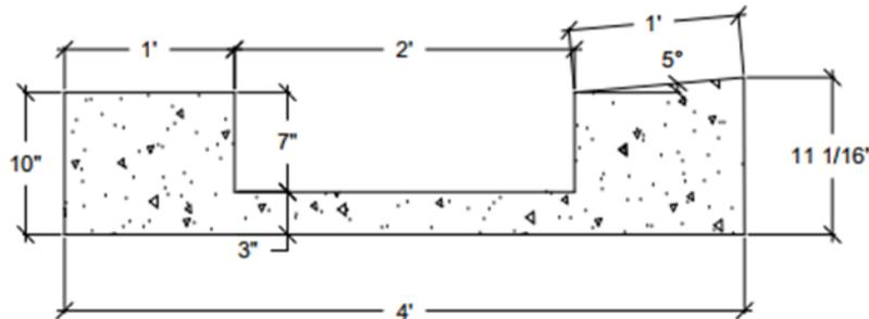
**Figure 25. UHPC-flowability test design modified cross-section**
