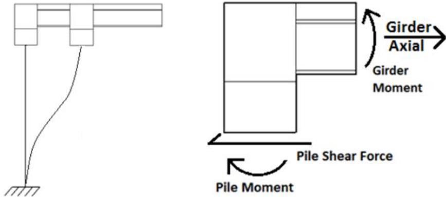
**Figure 53. Structural analysis for thermal contraction of bridge**
