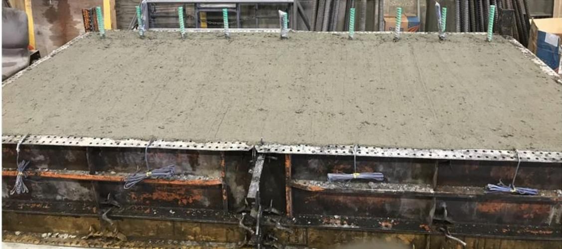
**Figure 29. UHPC joint pile cap cast in concrete**
