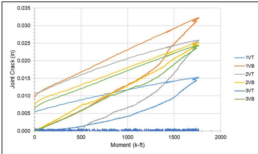
**Figure 60. Crack width versus moment due to vertical load**
