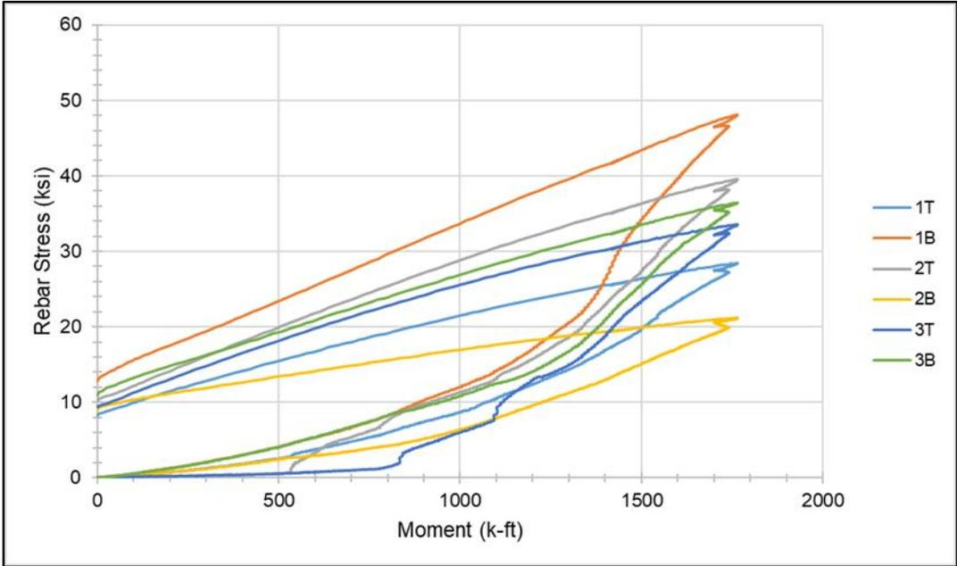
**Figure 62. Tension reinforcing bar stress versus moment due to vertical load**
