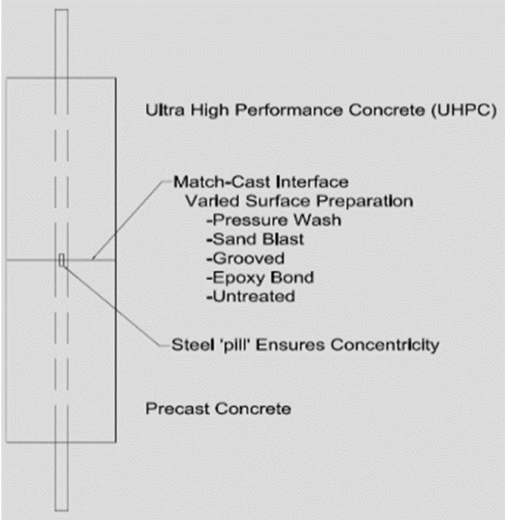
Figure 7. Direct tension test specimen
