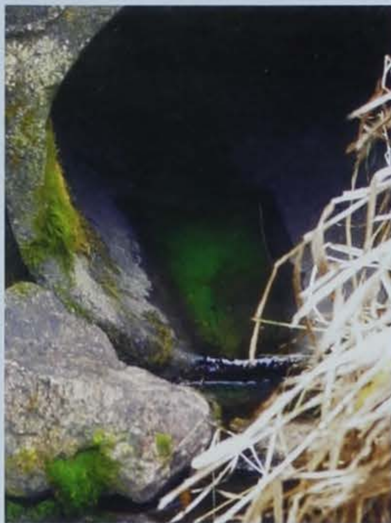
Green biodegradable dye helped traced the miles-long underground connection between tile inlets (above) and tile outlets (right) that flow into the stream.
