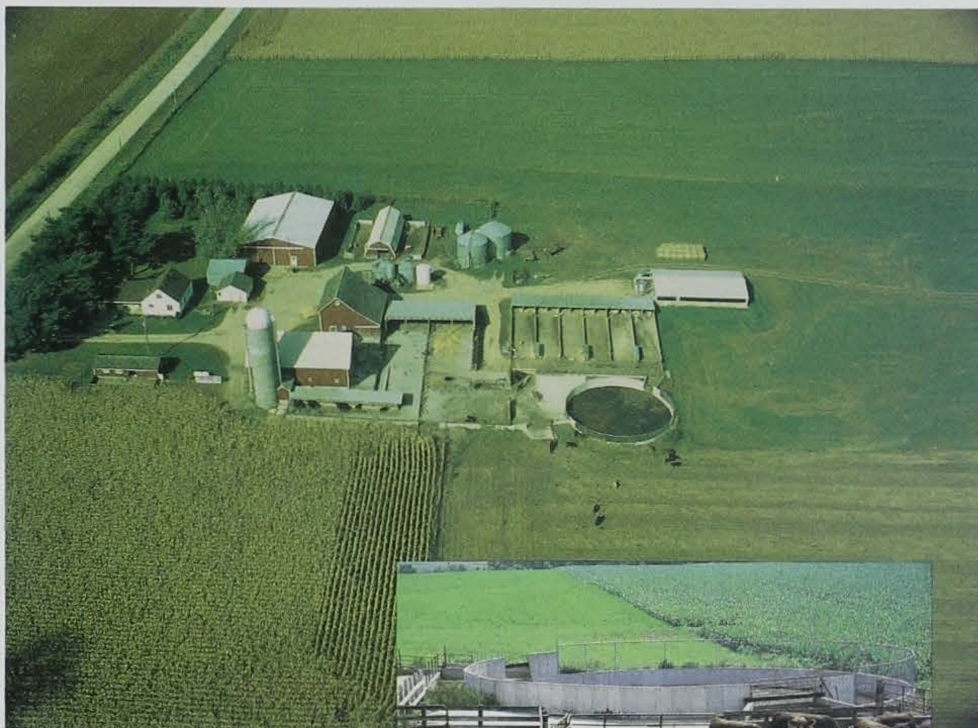
▲▶ The Trumm demonstration farm, concrete walls and planks settle out the solids while the liquid runoff flows to the storage pit for land application during the spring and fall.
