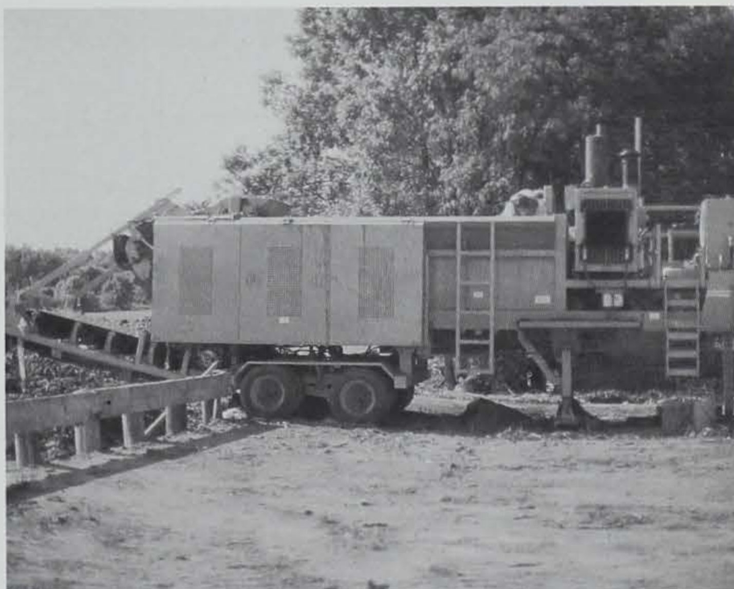
▲ At Organic Technologies Corp. near Van Meter a windrow turner (top photo) is used to stir the compost pile to circulate more air into the piles.
