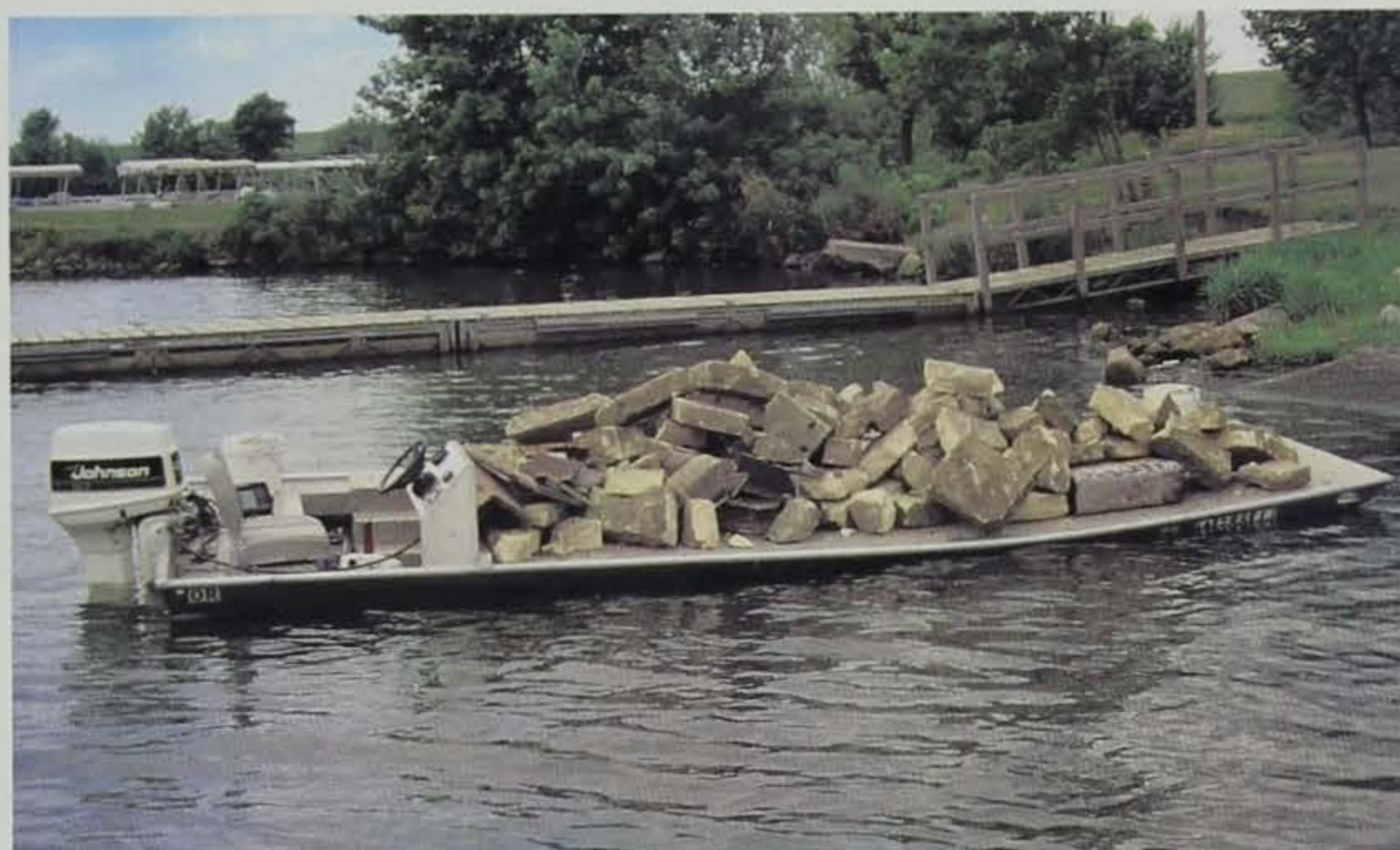
▲ Custom-built boat with a flat work deck is used for hauling rock to create reef habitat.
