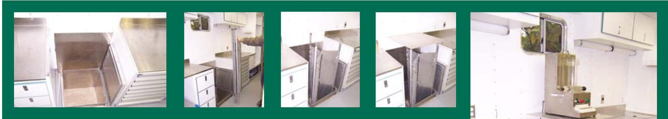
*AVA setup procedure in the PCC Center Mobile Concrete Research Lab: convert counter, remove floor portal door, lower weather shield through the floor portal, place three-legged stand on the ground protected by weather shield, place deck on top of stand, place AVA on top of deck.*
