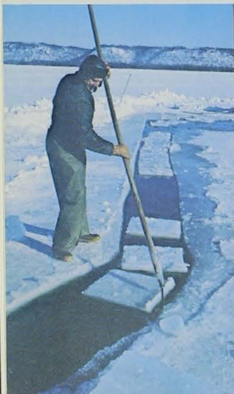
Above: Harvesting ice on the Mississippi River at Guttenberg. 150 lb. cakes of ice are guided with pike pole to elevator ramp for loading on truck. Below, left: Pike pole, spud bar, ice tongs and hand saw.
