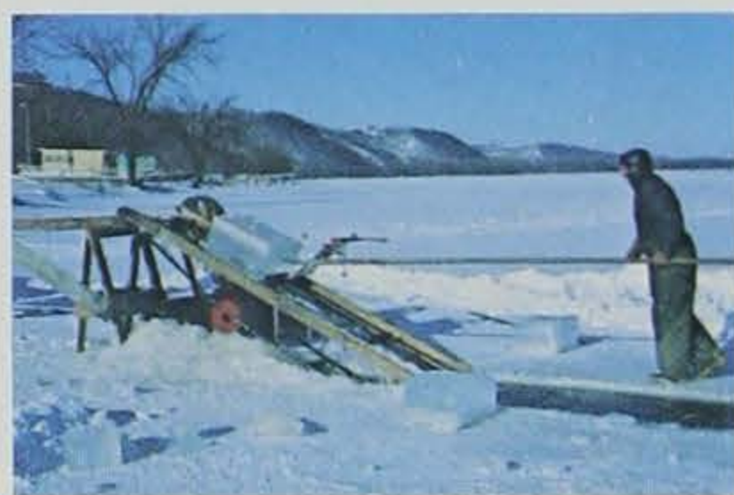
Above: Harvesting ice on the Mississippi River at Guttenberg. 150 lb. cakes of ice are guided with pike pole to elevator ramp for loading on truck. Below, left: Pike pole, spud bar, ice tongs and hand saw.
