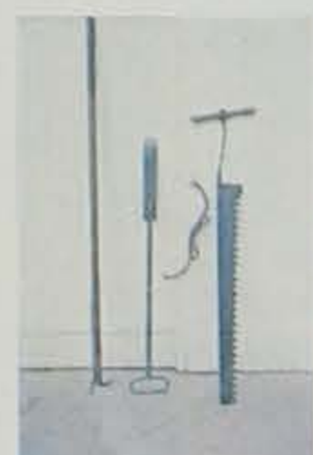
Above: Harvesting ice on the Mississippi River at Guttenberg. 150 lb. cakes of ice are guided with pike pole to elevator ramp for loading on truck. Below, left: Pike pole, spud bar, ice tongs and hand saw.
