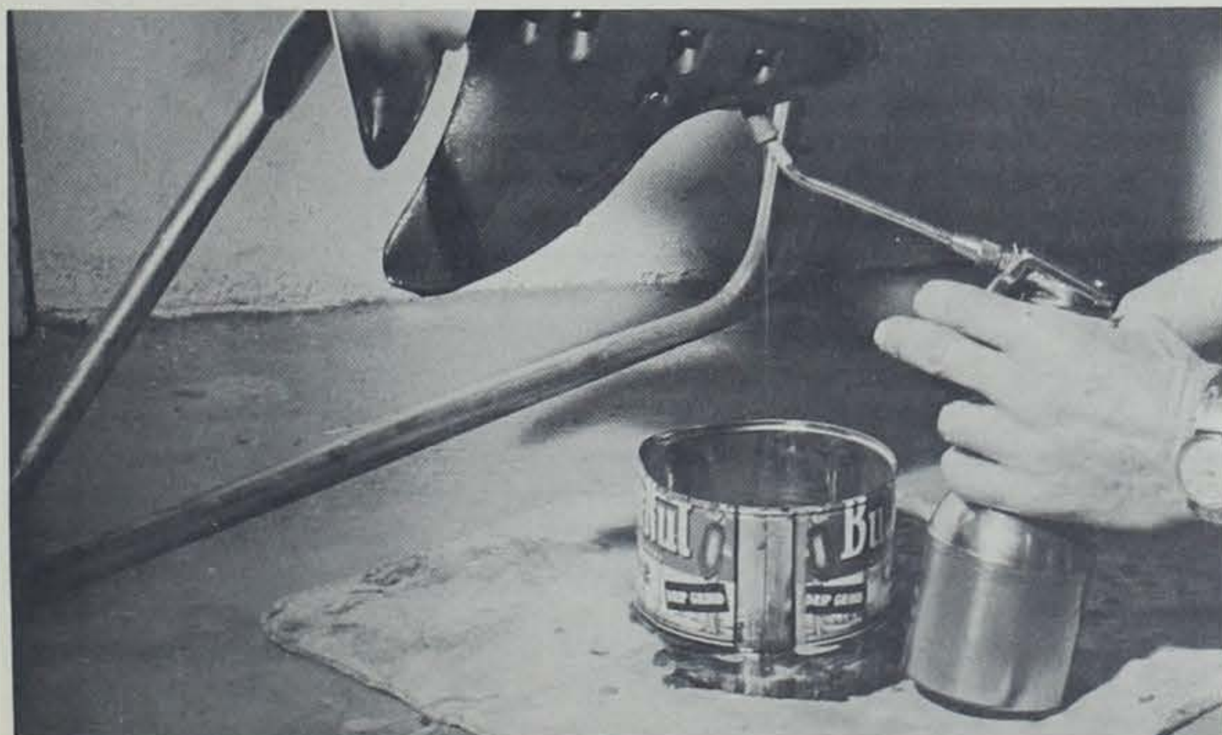
Drain lower unit in the fall and refill with oil (as shown) in the spring.
