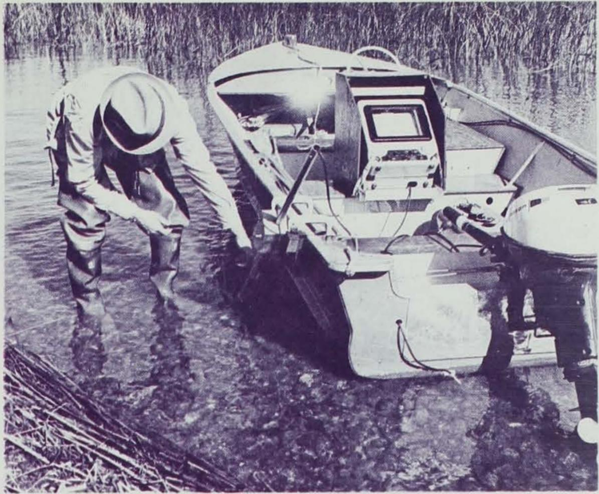
Boat equipped with fathometer and adjustable transducer.
