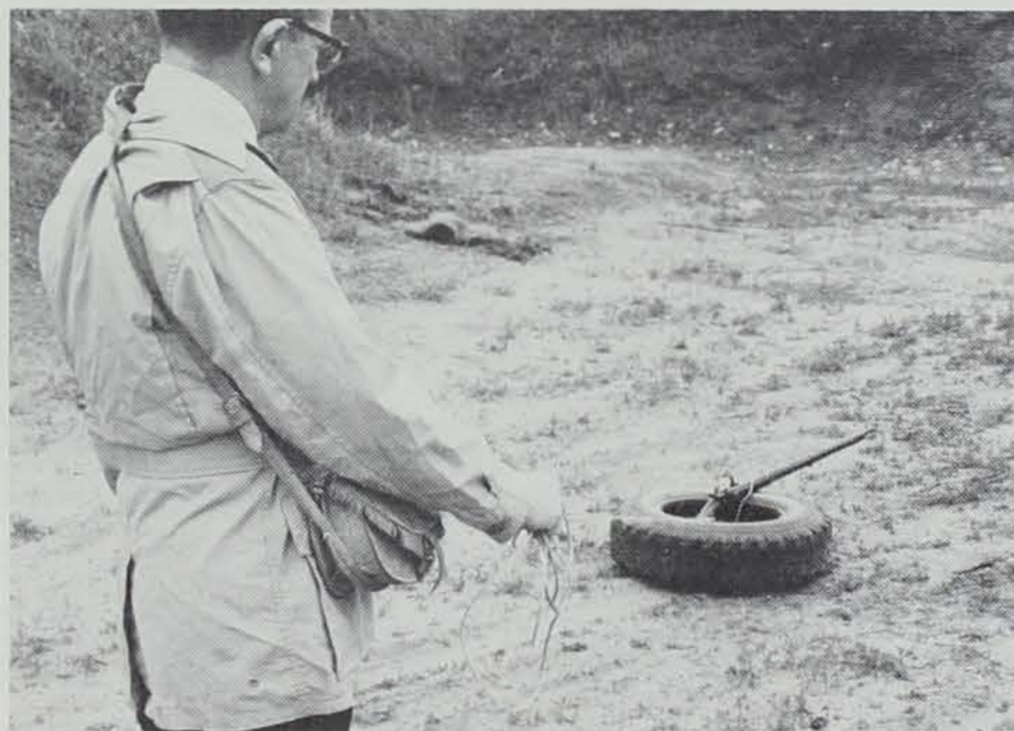
Mounting the piece on an old tire and firing from remote control is a sensible way to safely test fire it.
