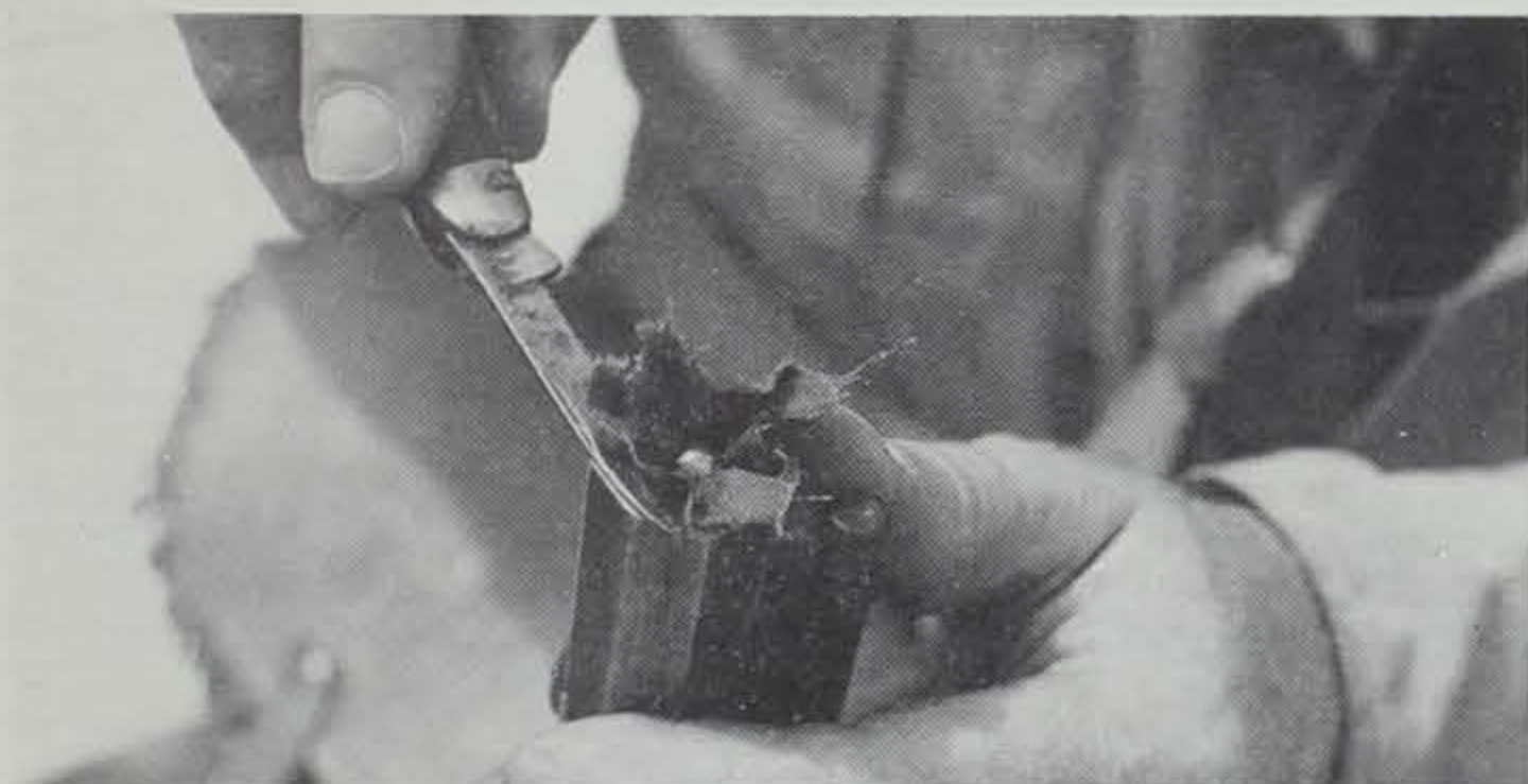
The ball is wrapped in cloth, placed flush with the muzzle, and then the excess cloth is cut away.
