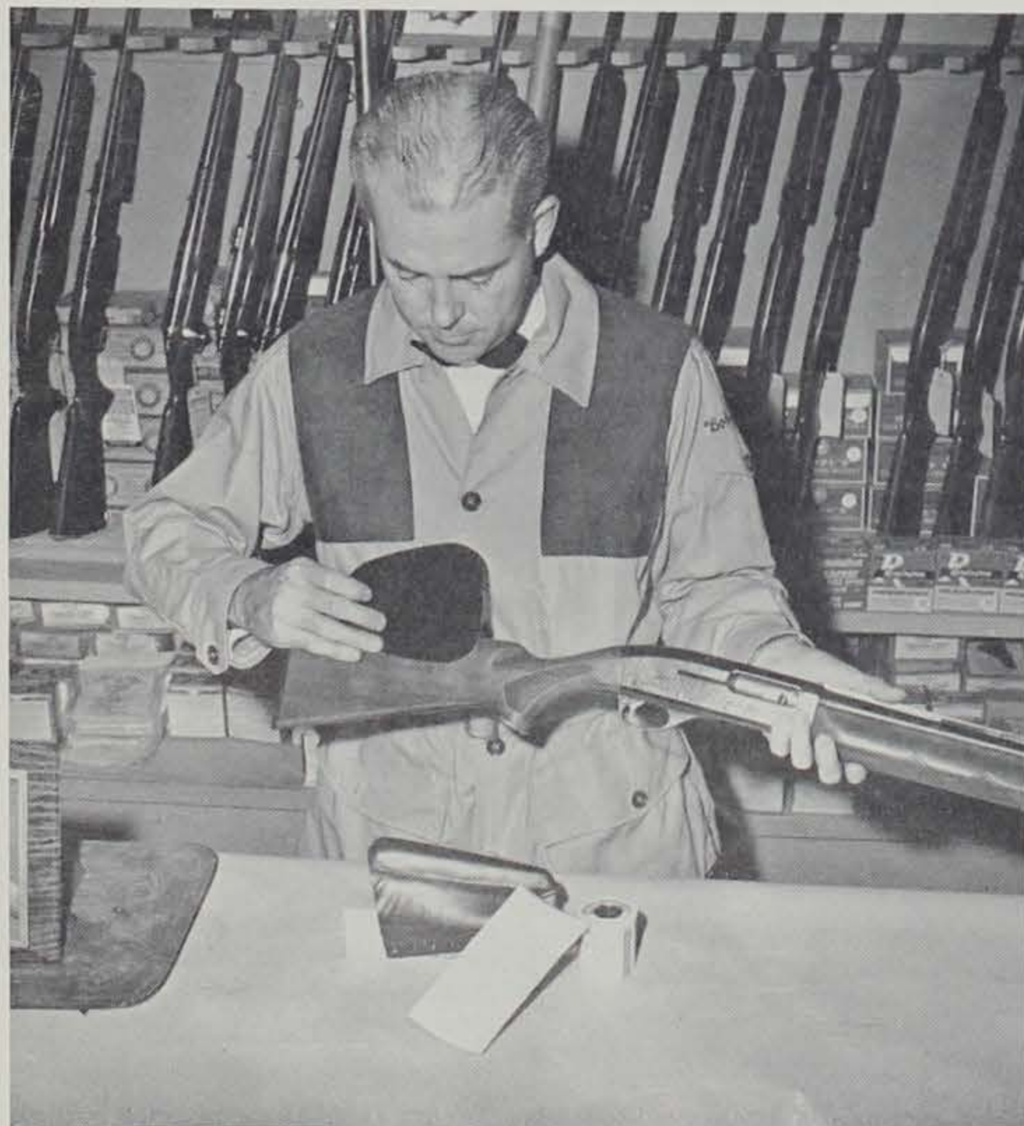
There are several ways to raise or fatten the comb. Shown are self-adhering comb pads, lace-on pads, and adhesive tape.
