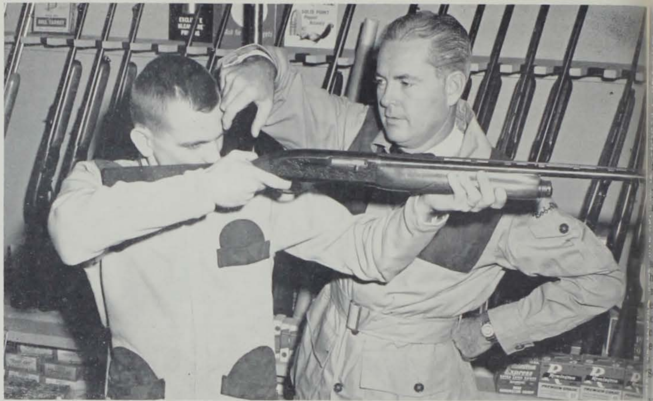
The measurement that indicates correct pull or stock length is the distance from the thumb knuckle to the nose.
