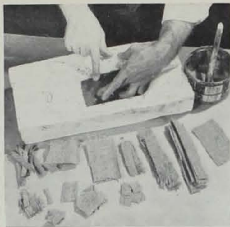
Make the strips fit before gluing and save a lot of trouble later. The first strips should be big and well soaked with glue.
