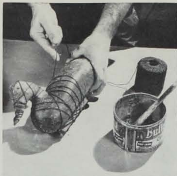
After applying a smooth thick coat of glue to both edges, wrap well with cord and make sure it lines up.
