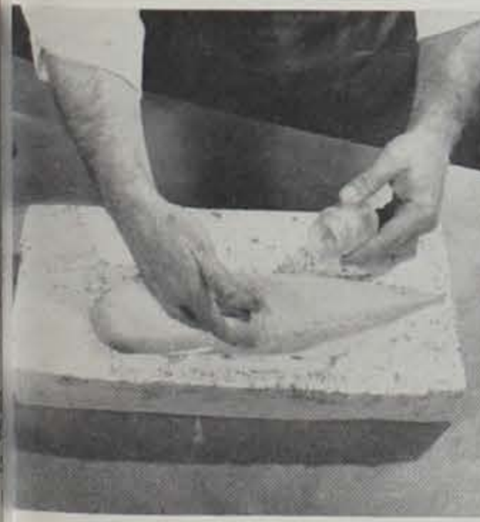
To facilitate removal of the built up model, grease the inside of the mold.
