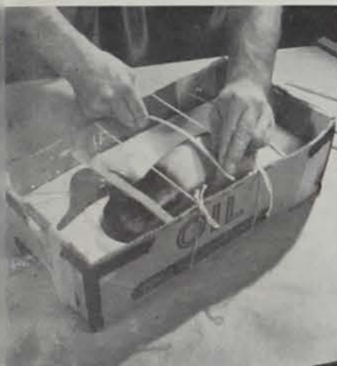
Wood is buoyant in the liquid plaster, so wooden strips are used to hold the box down to the pencil line. String maintains the shape of the box.
