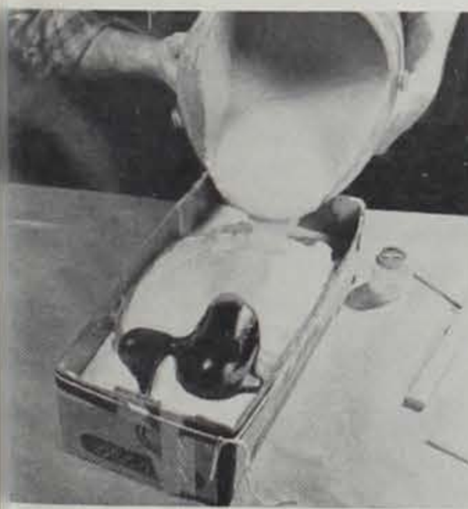
After greasing the face of the bottom mold of the decoy again, the top half can be poured. Plastic bucket is handy.
