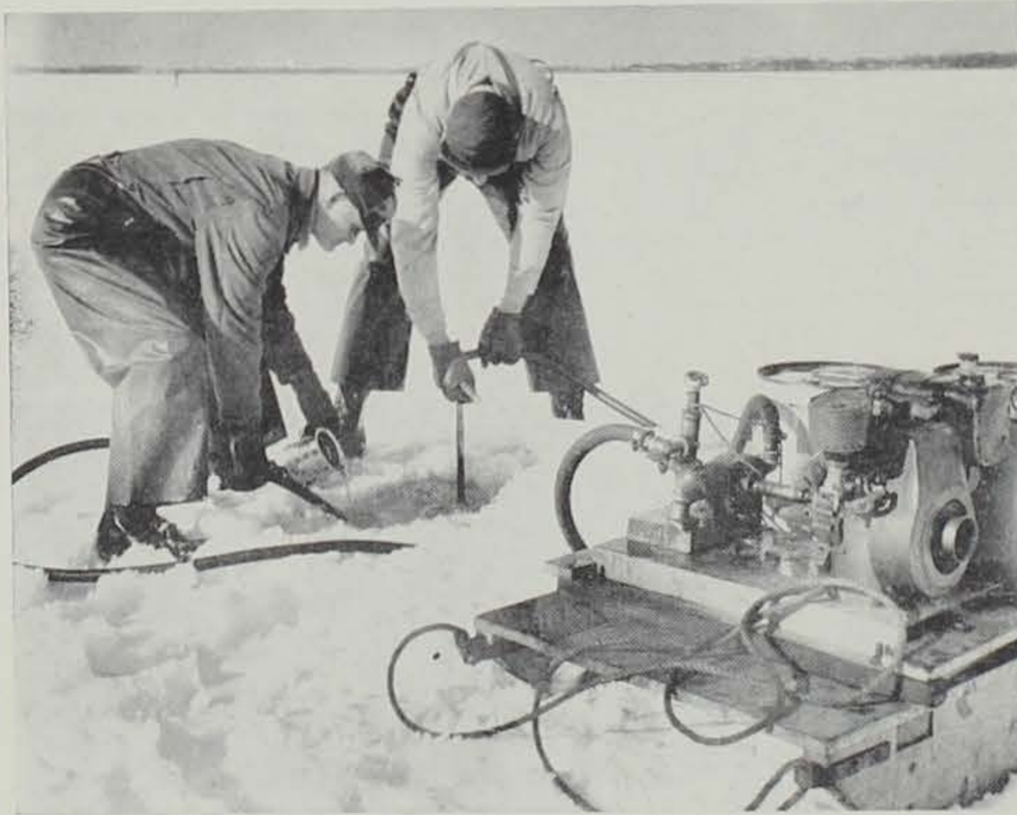
Pouring toxaphene into the water next to the mixing nozzle. As the water and chemical is drawn up through the pump in the foreground it mixes and is then sprayed out through the "T" handled hose. With such force behind it, the chemical effectively treats an area nearly 400 feet around the hole.
