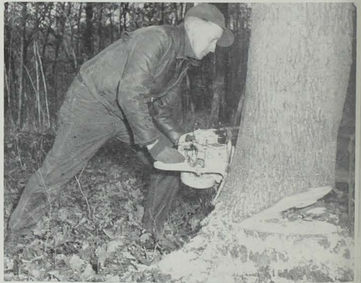
A modern chain saw makes quick work of a mature tree that's already past its prime. Heart rot has begun, reducing total board feet and the value of the log. An earlier cutting on the advice of a trained forester would have brought a better price.
