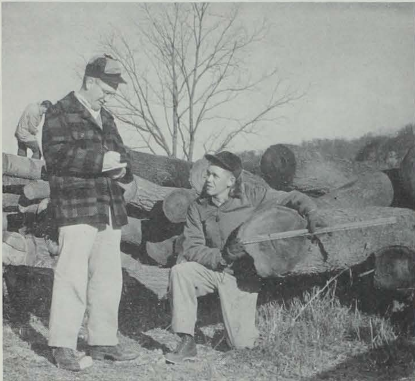
By measuring log diameters and lengths, foresters can estimate the total volume of a tree harvest. District Forester Gene Hertel, now head of the State Forest Nursery, jots down calculations for the volumes of oak logs.
