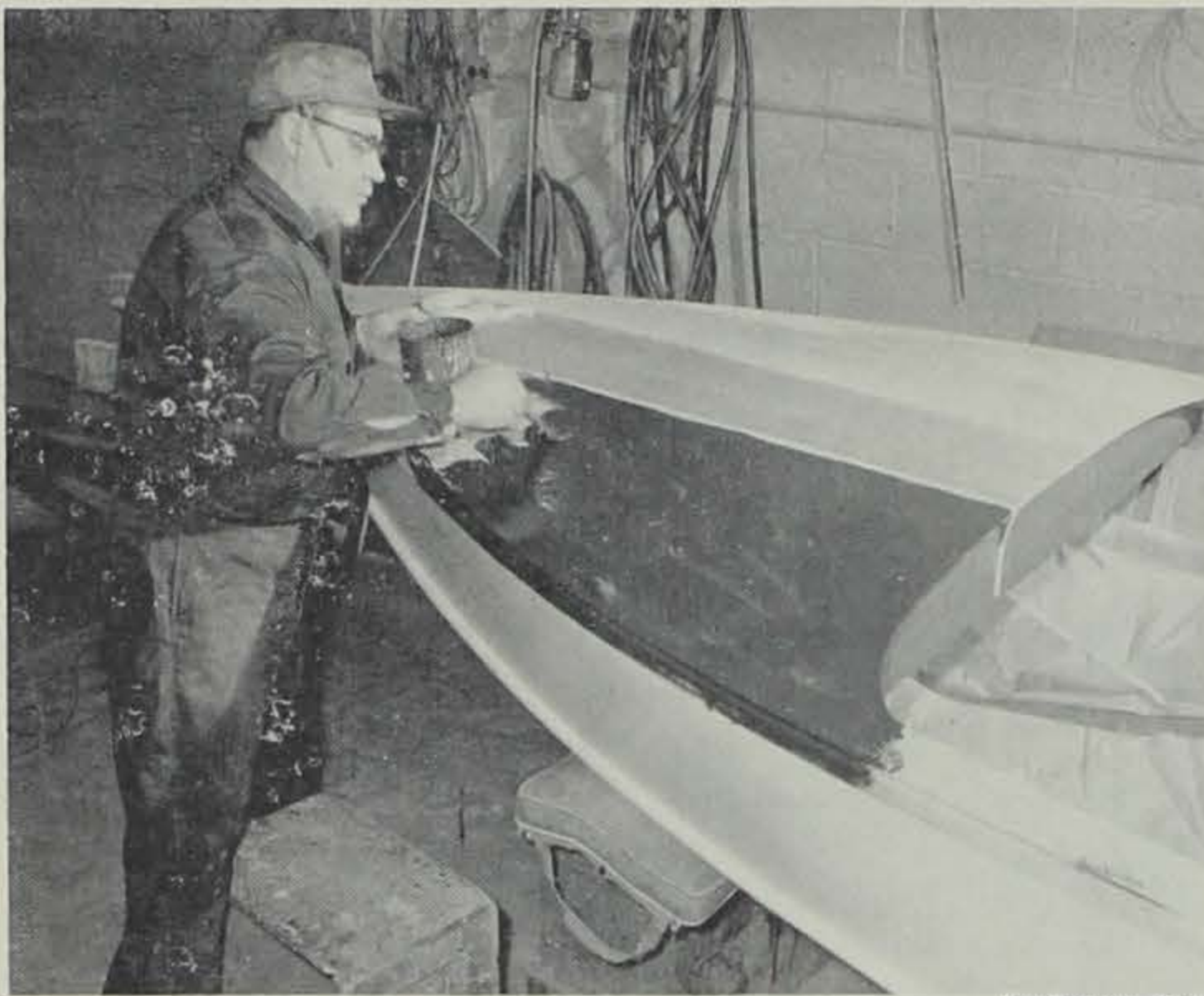
An expert job of boat finishing will last for years. Herman Leinen, builder for a Des Moines boat firm, carefully stains a mahogany hull, using masking tape to define a center plank.
