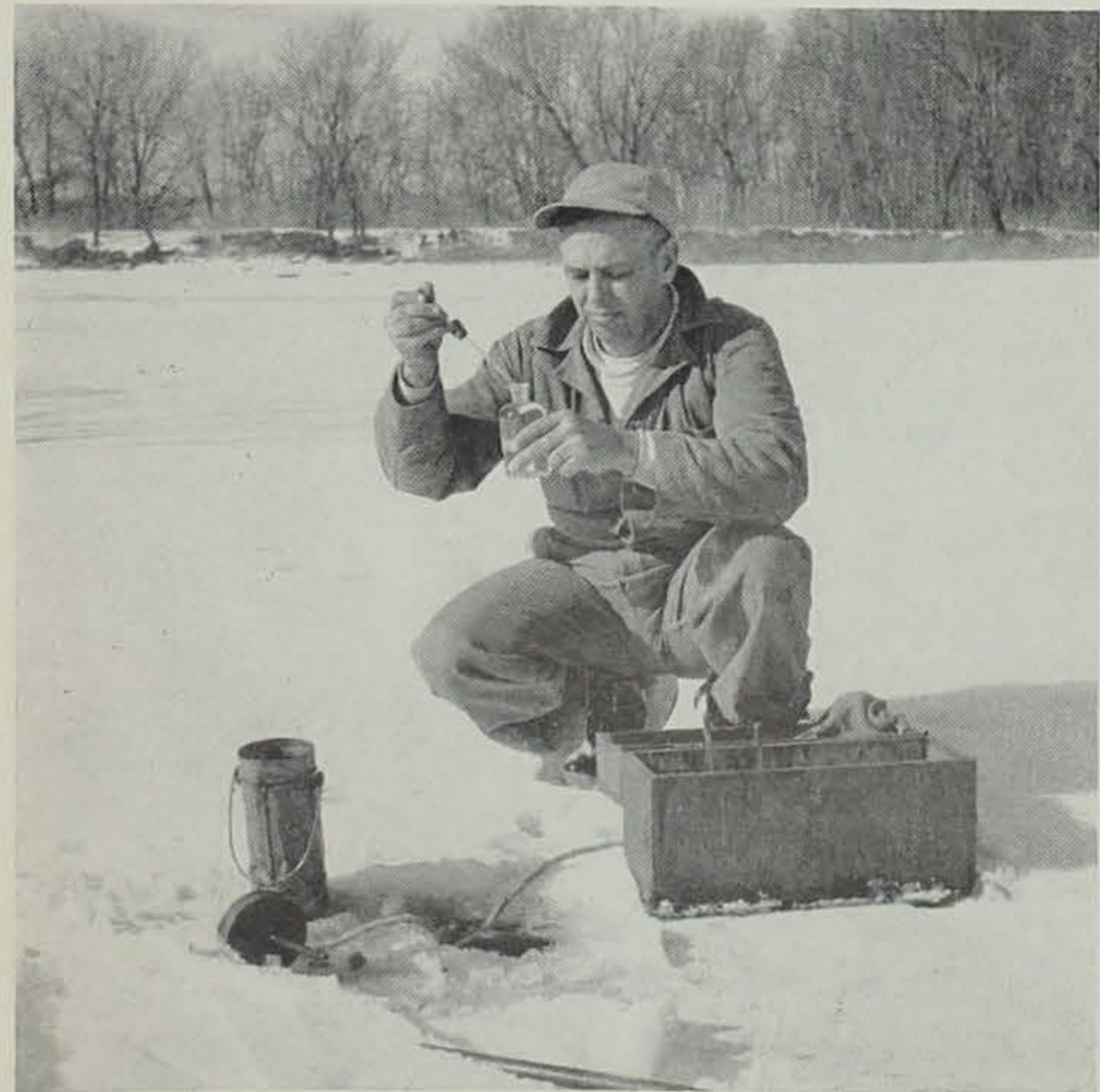
Jim Sherman Photo. Hundreds of water samples were taken last winter to determine dwindling oxygen supplies. Fisheries biologists like Harry Harrison were in the field almost constantly.
