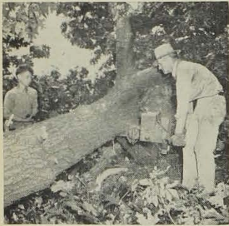
Inverted bucking or sawing from the bottom side to the top side is almost impossible with a cross-cut saw. It is easily done with a chain saw. This Disston-Mercury saw will make the cut in about 30 seconds.—Farm Forester Photo.
