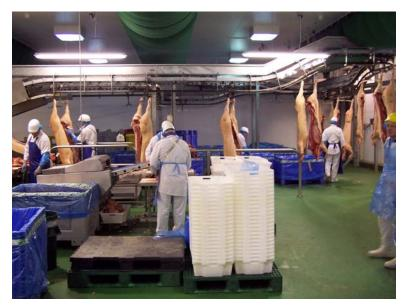
FIGURE 12. Carcass splitting and quartering
