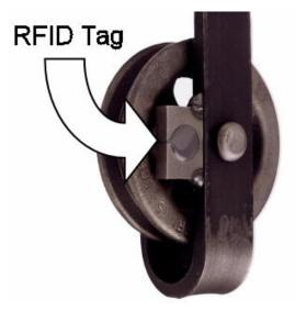
FIGURE 9. Gambrel radio frequency identification assembly
