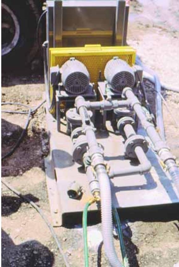
Figure 2. Mixing unit for combining concentrated latex with water prior to dispensing.
