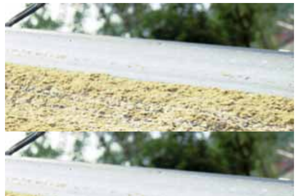
Figure 4. Coated aggregate moving up conveyor.
