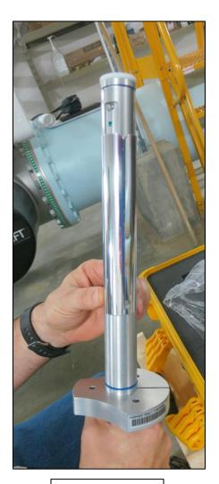
UV Light used for Cryptosporidium Inactivation
