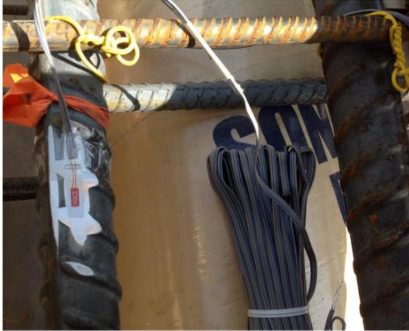
**Figure 14. Gage installation on reinforcement**
