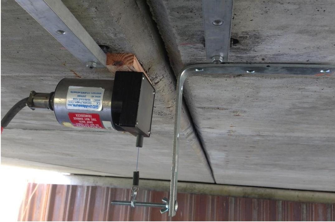
**Figure 33. Relative displacement gage setup**
