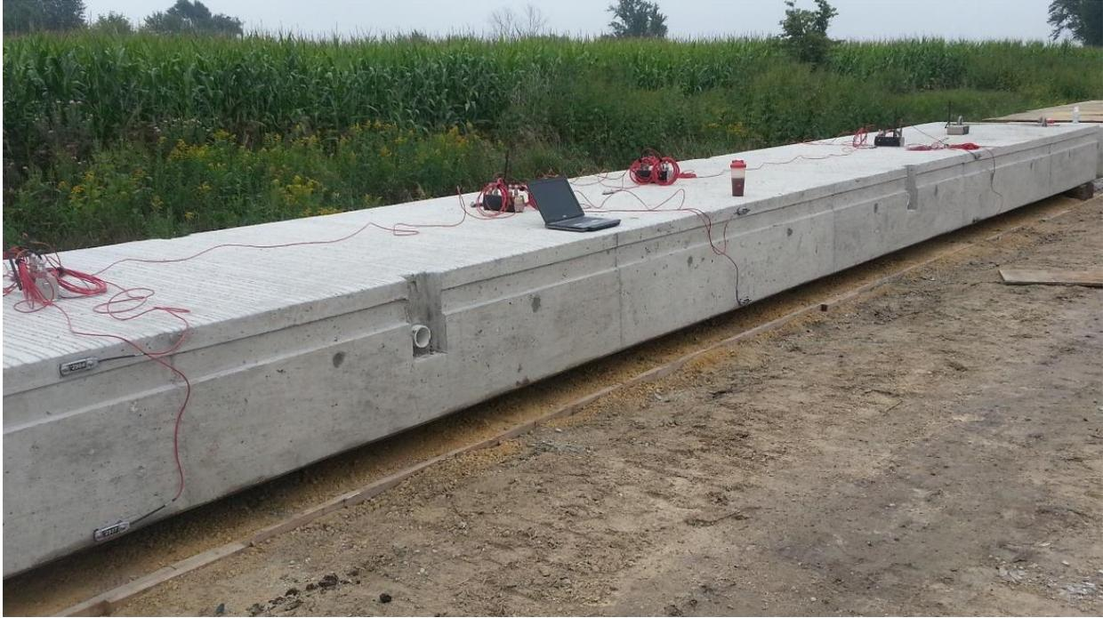
**Figure 20. Installed strain gages and data collection system for lift/move**
