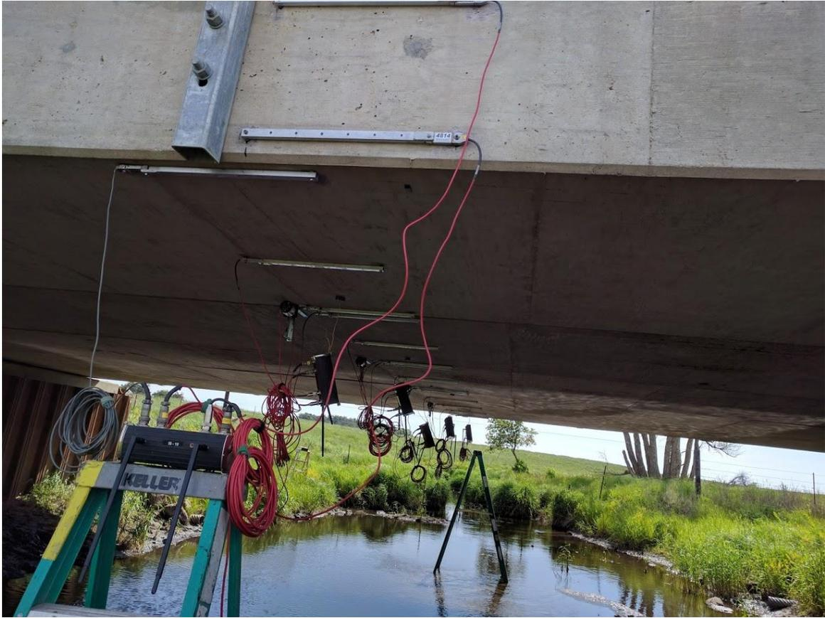
**Figure 32. Instrumentation mounted on the bridge**
