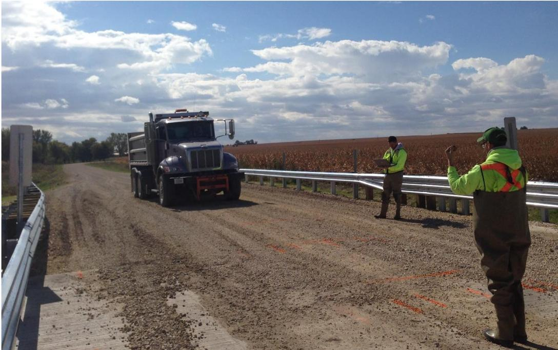
**Figure 34. Live load testing on the bridge**
