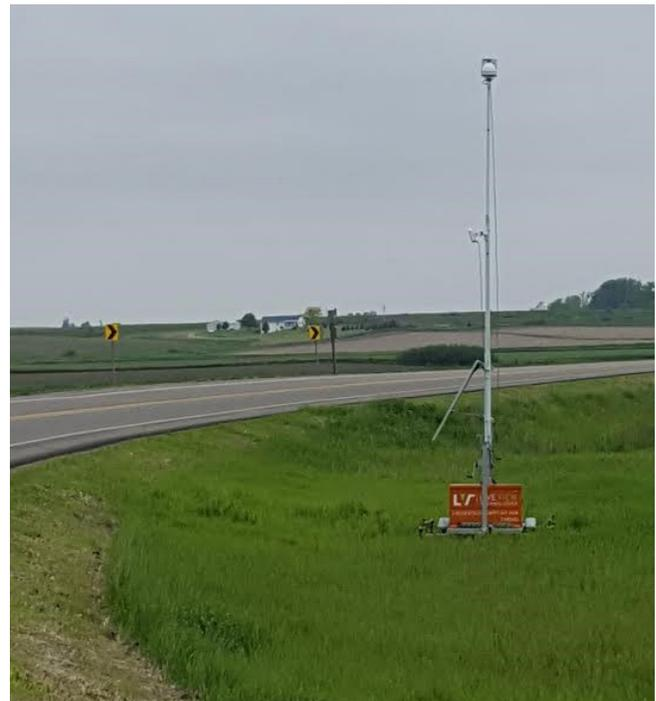
*Data collection trailer components, including a 360° camera, Wavetronix sensor, and solar panel*
