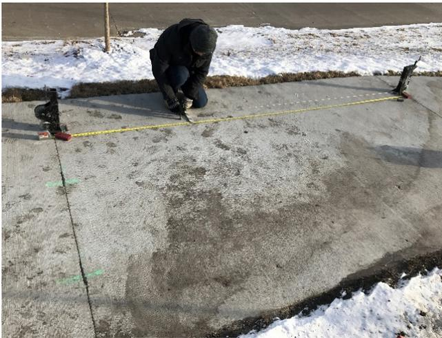
*Measurements to monitor deflection/slab surface profile over time*
