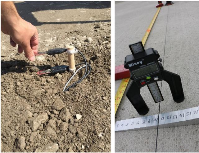
*Installation of sensors at the top and bottom of the slab before it gets placed (left) and digital height gauge used with portable device for profile measurements (right)*
