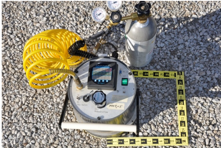
Figure 22. In situ APT setup for determination of saturated hydraulic conductivity
